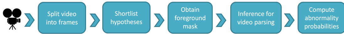
Figure 4.1: The pipeline of the sequential video parsing. To parse a single video frame, a shortlist of object hypotheses is created, such that they are sufficient for explaining a foreground mask. By probabilistic inference, video parsing selects a subset of hypotheses that are necessary for explaining the foreground, and simultaneously matches them to normal training samples. Probability of abnormality is eventually calculated for all selected hypotheses and foreground pixels.
