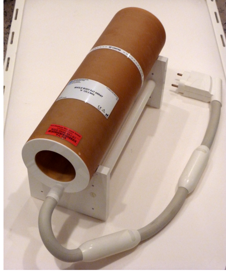
Figure 3.2: Eight channel receive-only volumetric rat array manufactured by Rapid (Rapid Biomedical GmbH, Rimpfing, Germany). The coil allows to image small animals on a whole-body scanner.
