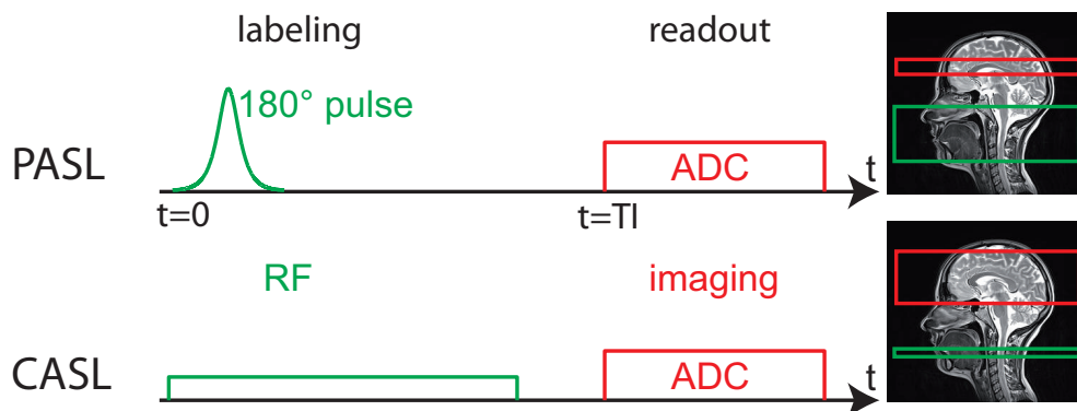
Figure 2.17: Illustration of the two basic ASL techniques: pulsed and continuous arterial spin labeling. While for pulsed ASL the labeling is performed with a short inversion pulse, CASL employs a continuous RF application with a low amplitude. Usually, the labeling region of CASL is smaller compared to the inversion slab of PASL. Both methods comprise an imaging module that starts at a time t = TI after the labeling has started. Independent of the method, this can be a 2D, 3D or a multislice readout. The sketch does not show the control phase of the ASL experiments. Figure adapted from Gregori [2009].
