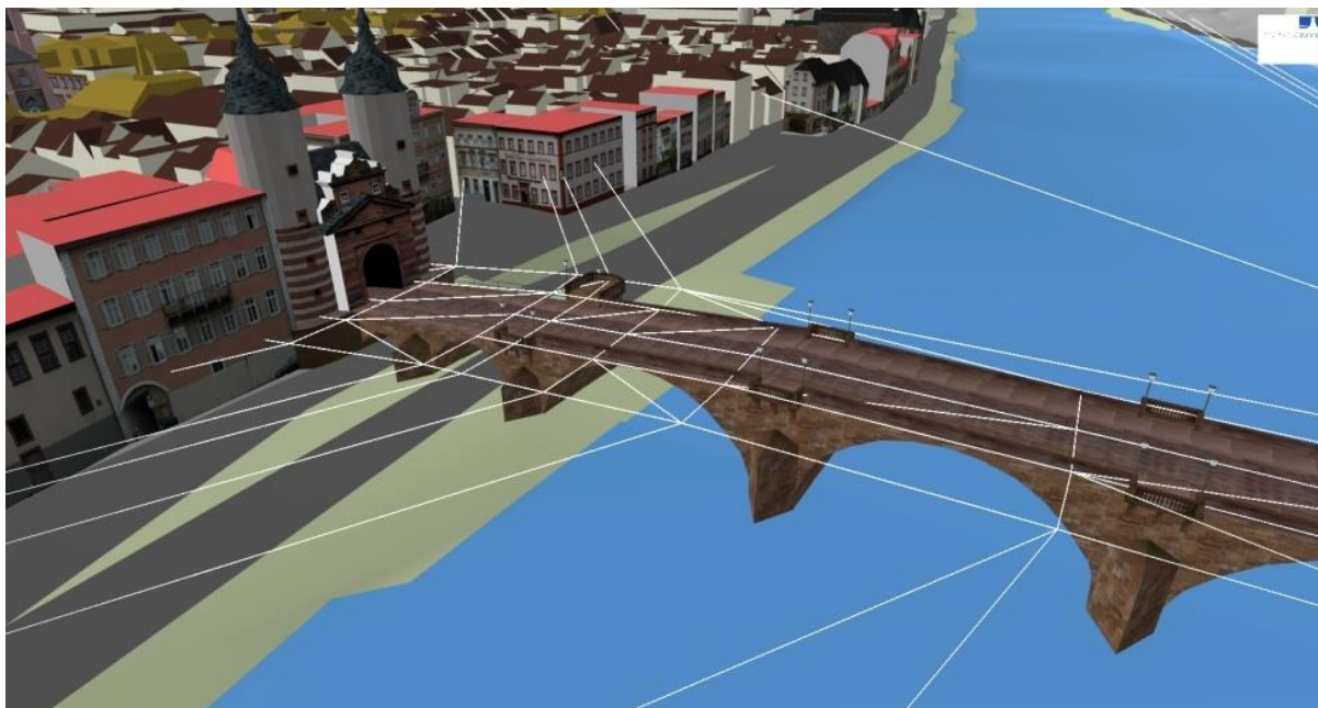
Figure 44: For bridges and tunnels a second surface model is used in addition to the usual terrain (here rendered as wireframe model).
