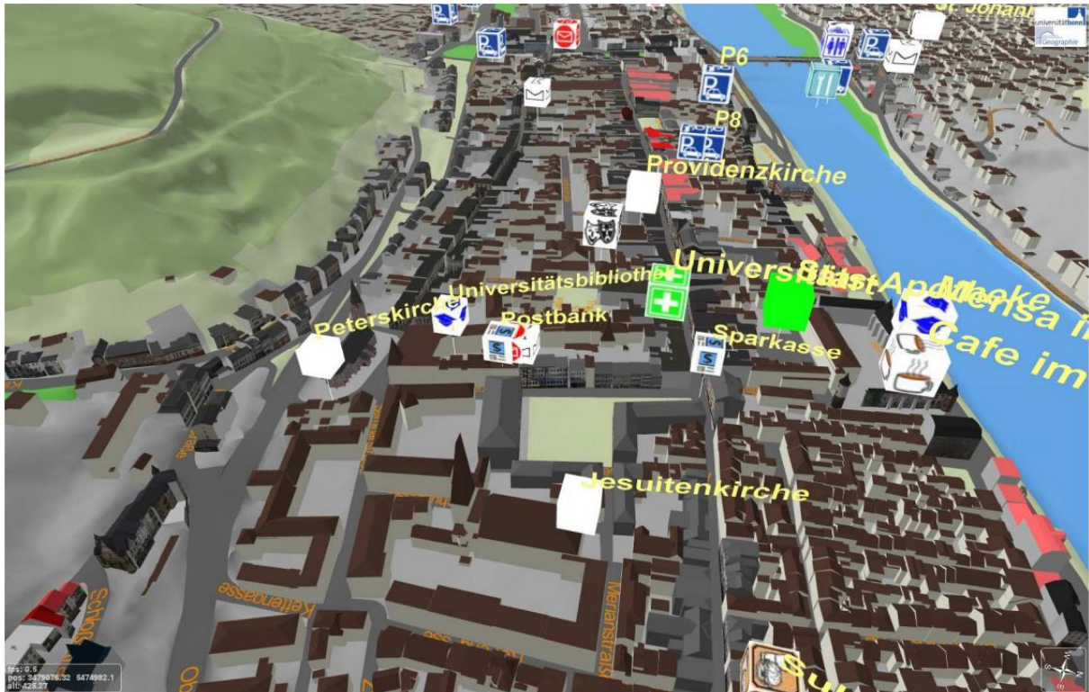
Figure 53: Using the OpenLS Directory Service (local search for POIs) based on OSM data together with official city data – the case of www.heidelberg-3d.de.
