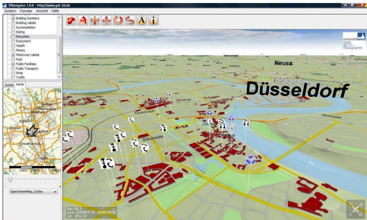
Figure 58: Web 3D Service for Germany based on user generated geodata (OSM) and SRTM. Landuse, buildings and POIs generated from OpenStreetMap. The range of OpenLS services available from GDI-3D.de offering OSM data in distinct ways is available also in this application from the integrated client XNavigator. Example: Düsseldorf
