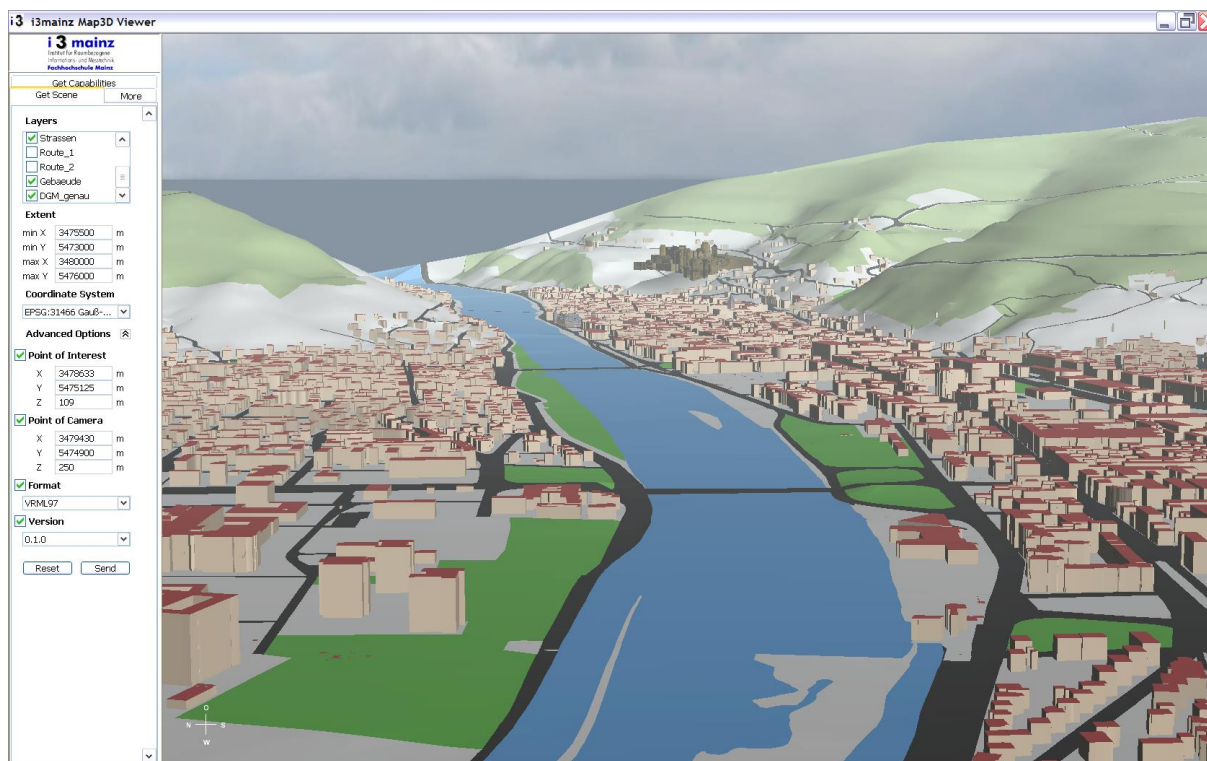
Figure 27: Screenshot of the final Web 3D Map client. The software runs as Java Webstart application and includes a custom Java3D viewer. Parameters for the OGC GetScene request can be set on the left panel, which include layers, spatial extent, coordinate system, POI, POC and others. Data courtesy of Land Surveying Office City of Heidelberg.
