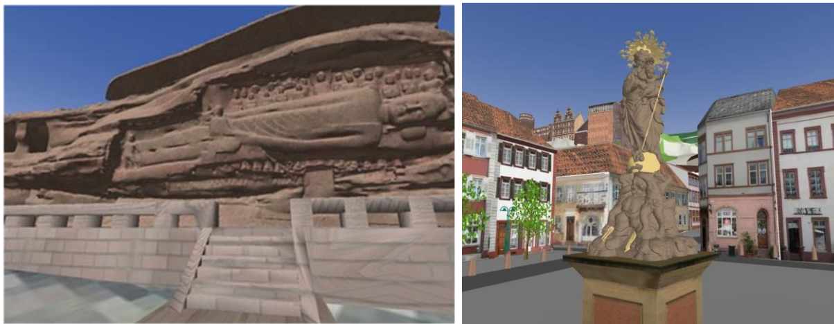
Figure 14: Data from terrestrial laser scanning embedded as scene graph objects and streamed through a Web 3D Service. Left: cultural heritage site in Sichuan, China. Right: Marienstatue in Heidelberg.
