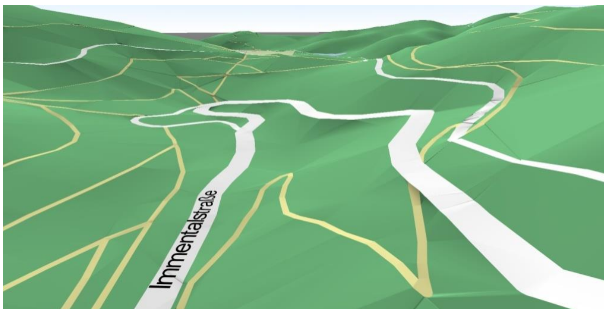
Figure 50: Some mountain roads integrated into the terrain and flattened. Major roads have a higher priority and have been flattened more than smaller forest tracks.
