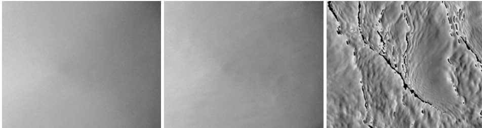
Figure 9.1.: Wave slope images measured with the ISG. Displayed is the alongwind slope component; the wind is blowing from the left.
