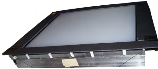
(b) Light source with acrylic diffusing screen.
