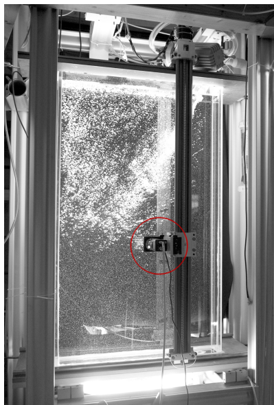
Figure 4.1.: Photograph of running bubble tank with illumination from below. Red circle marks a single camera for the bubble measurement setup.
