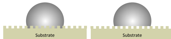
Figure 3.3.: Wenzel vs. Cassie model. The main wetting models aiming to describe the wetting of textured surfaces.
