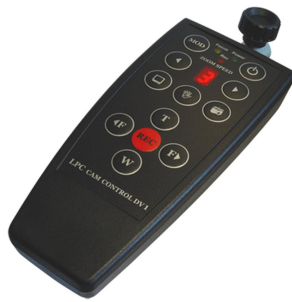
Figure 4.2.: The LANC controller synchronizing the cameras. The LANC controller purchased was used as an external synchronization and trigger device.
