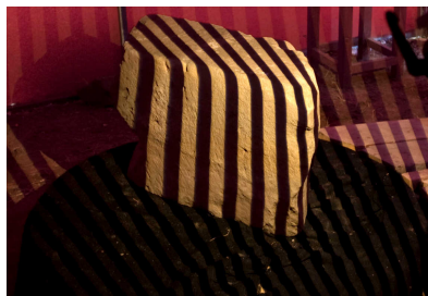
(b) A stone with the typical stripe pattern of the 3D scanner.
