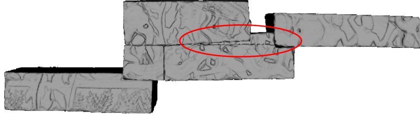
Figure 6.1: A solution with a high similarity score. The red ellipse marks a stone whose final position means to intersect with the other stones in the dataset. While this positioning can be rendered on a computer it is impossible in the real world. Therefore it has to be ensured that such infeasible solutions are sorted out.
