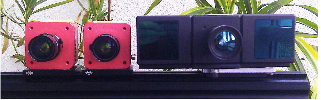
Figure 3.2: Camera setup. The stereo subsystem (Red cameras) consists of two Photon Focus MV1-D1312-160-CL-12 with Linos Mevis-C lenses at 25mm/1.6, 1312x1082px. The ToF camera (Black camera) is a PMD Tech Camcube 3, 200x200px .
