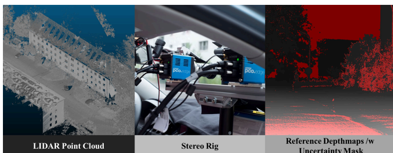
Figure 1.6: Reference Data with Uncertainty. Left: LIDAR point cloud used to generate stereo reference data. Middle: Stereo rig used for image acquisition. Right: Depth maps with a mask excluding pixels beyond a certain uncertainty.
