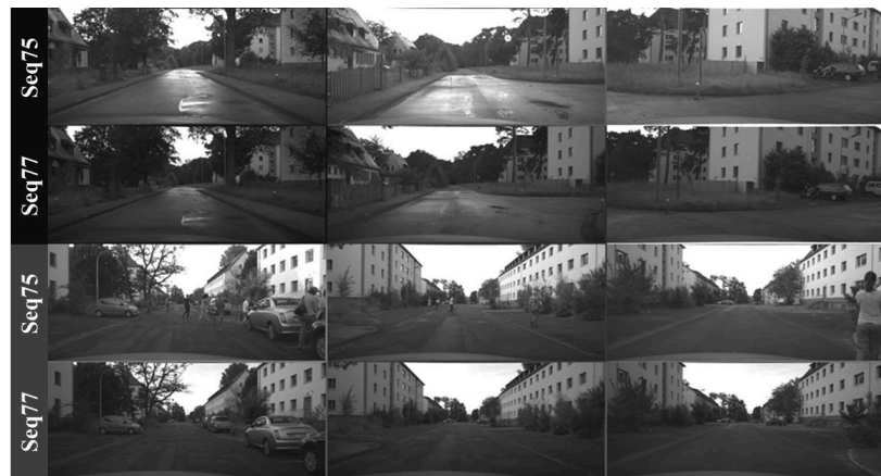
Figure 4.20: Examples of bootstrap alignment between sequence 77 and 75. Top of image pair: Sequence 75 that is not registered. Bottom of image pair: Registered sequence 77. Results shown from top left to bottom right for frames 62, 1779, 2200, 4108, 5928 and 7004. The other images show similar performance. Visual inspection of these image pairs suggest a relate pose difference bound by 2 - 5 meters.
