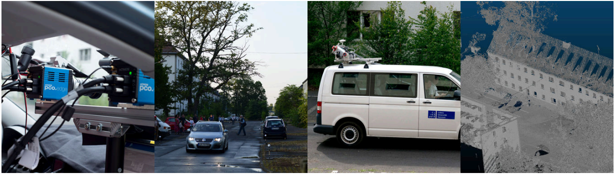
Figure 4.4: Experimental Setup. From left to right: Stereo rig, set photo, LIDAR mounted on car and resulting data. A video showcasing the collected data can be found at http://hci.iwr.uni-heidelberg.de/Benchmarks/document/StereoErrorBars
