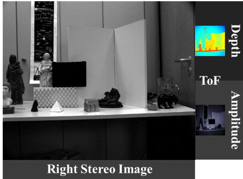
Figure 3.4: Input: Time of Flight data (200x200), One of the stereo images (1312x1082). Images are depicted to scale.
