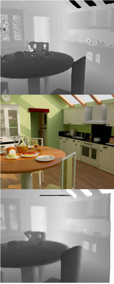
Figure 3.6: Illustration of reprojection and interpolation step on synthetic data. Top: ToF range image (dark is near, bright is far). Middle: Left color image. Bottom: Reprojected depth image. Note the fattening occurring on the right-hand side of object silhouettes. The confidence measures in the next section account for this. N.B. This depth image has to be converted into a disparity map in a subsequent step.
