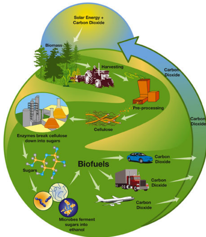
Figure 1.3: Schematic representation of the production cycle of biofuels [15]
