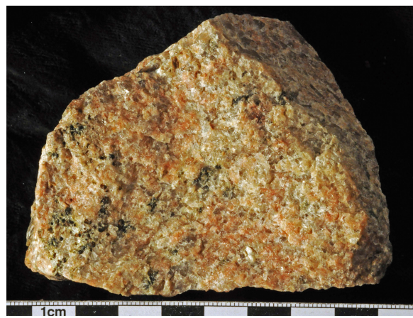
Fig. 2.9: Migmatite with mafic minerals partly concentrated in some areas (ARG 12-10).
