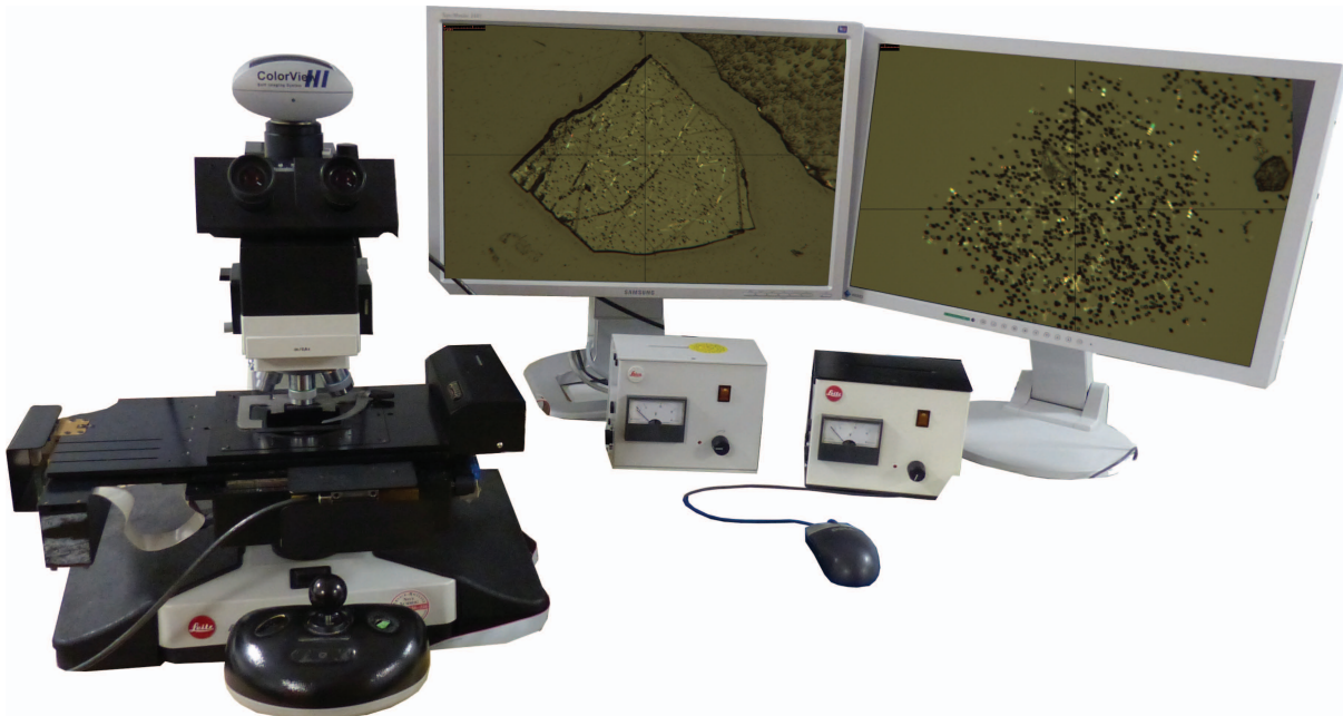
Fig. 4.1: Leitz FT station for data acquisition.
