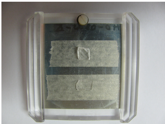
Fig. 12.1: Two calcite crystals, which were used for the luminescence test with an energy of 11.1 MeV/u.
