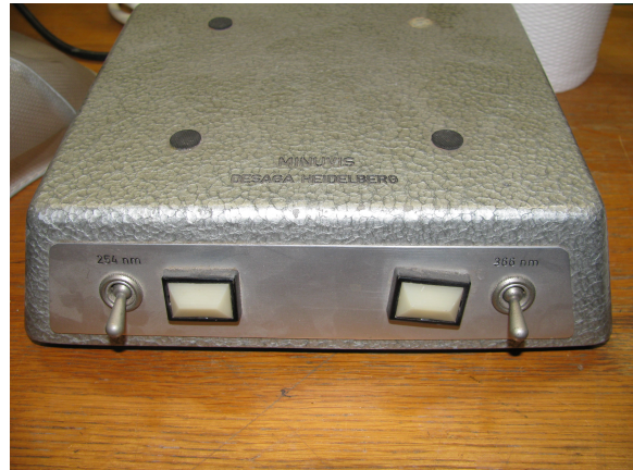
Fig. 12.6: UV-lamp used for the UV-experiments. It provides two different wavelength: a short wave UV-light at 254 nm and a long wave UV-light at 366 nm.
