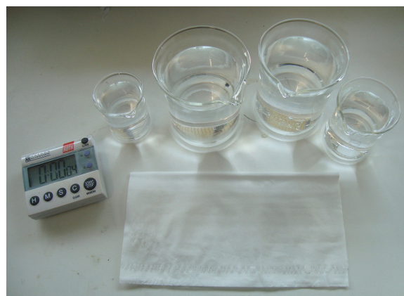
Fig. 3.17: Setup for the etching experiments. From left to right: stopwatch, etching solution, 2x pur. water, ethanol.
