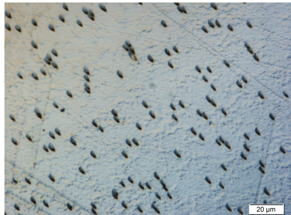
Fig. 6.5: Etch pits on the formerly coated sample. 0.91 % \text{HNO}_3 for 1 s was able to display the etch pits. ( 1 \times 10^6 ions/ \text{cm}^2 , 11.1 MeV/u, ^{197}\text{Au} )
