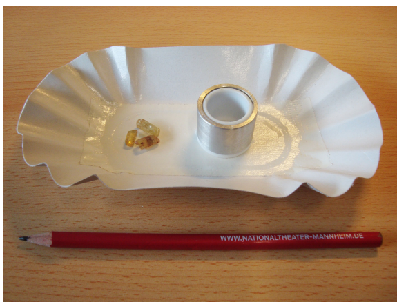
Fig. 4.3: Dish with double sided duct tape. On the left are apatite crystals (for better contrast). To embed these crystals, the form on the right is glued to the duct tape over the crystals and filled with epoxy resin.
