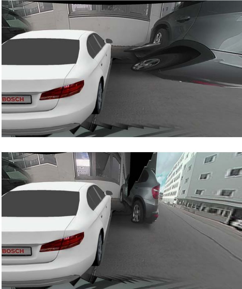
FIGURE 6.10: Example of dynamic projection surface adaptation - Scene 2. Based on occupancy grid information a depth extractor is applied as presented in Section 6.2. The effects of the adaptive mesh can be observed on the gray vehicle, especially on the lower part of the main body and wheels. Without depth information the projection surface is set to its default shape, thus the car body and wheels are projected on the floor. On the contrary, with correct depth information, the walls of the surface approximate well the side of the car, providing a more intuitive representation. Top: default static mesh. Bottom: Adapted mesh.
