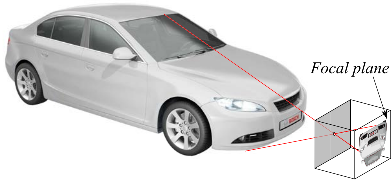
FIGURE 3.5: Pinhole camera model. The ideal pin-hole camera model assumes all light rays passing through a single common point and projecting onto a focal plane.
