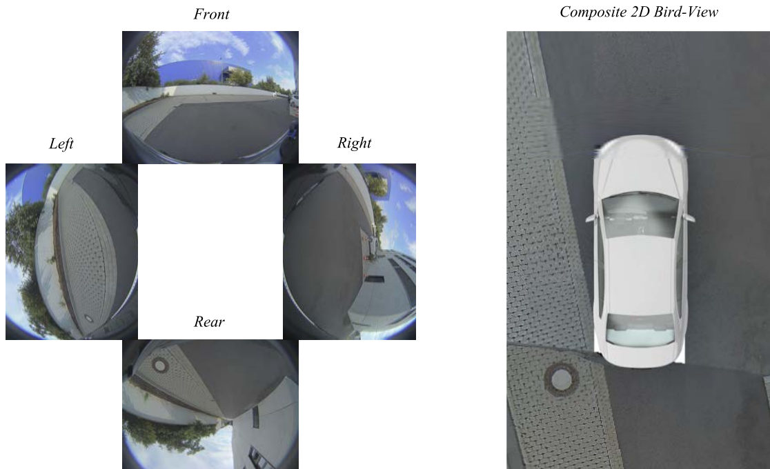
FIGURE 2.4: Bird-view composition from original fisheye images - Scene 2. Left: Original fisheye images as acquired by the cameras. Right: Composite view after projecting the images onto the ground plane.
