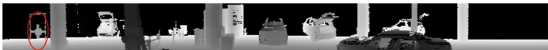
FIGURE 4.3: Example of rasterized depth map, as seen from the 3D LRF virtual center. In red: Target used for manual selection of keypoints. Taken from [Esparza et al., 2014c].
