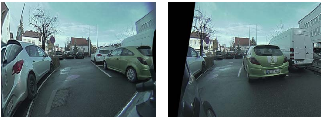
FIGURE 5.21: Example of traditional configuration prior to entering a narrow drive path or park space. The images correspond to the Front-Right camera pair, and are epipolar-rectified. The large parallax can be observed on the green vehicle. In particular, the side of the car offers a very different surface resolution to each of the cameras, which reduces the chances of correct keypoint matching.
