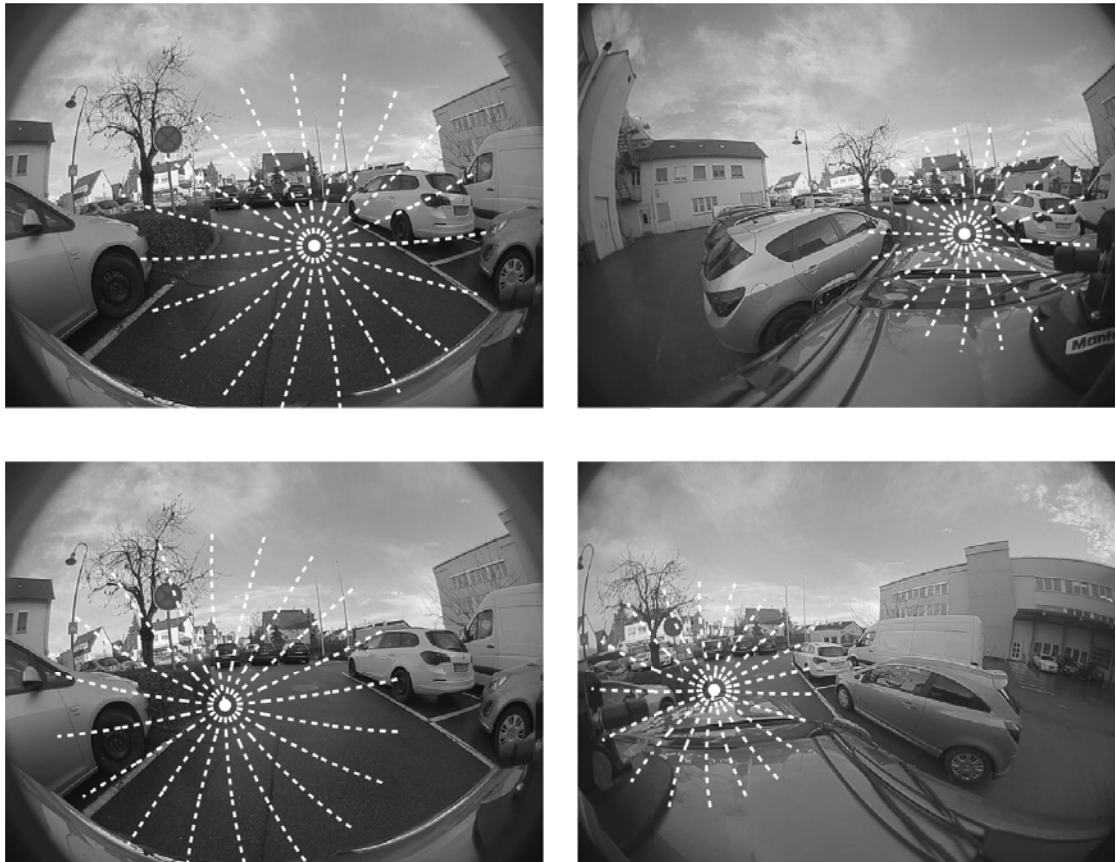
FIGURE 5.24: Epipolar lines on original fisheye images, for the camera configuration depicted in Figure 5.23. Top row: Front-UpperLeft camera pair. Bottom row: Front-UpperRight camera pair. Taken from [Esparza et al., ].
