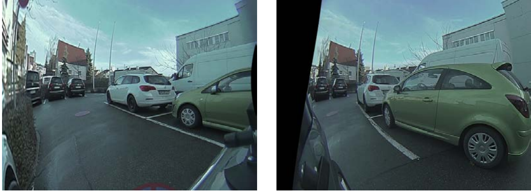
FIGURE 5.22: Example of traditional configuration inside a narrow drive path or park space. The images correspond to the Front-Right camera pair, and are epipolar-rectified. The lateral side of the white vehicle is observed from very different perspectives by both cameras. This complicates the search of correspondences.
