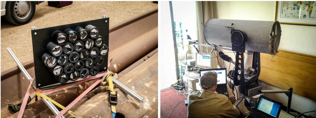
(a) Retro reflector array consisting of 24 single reflectors (each 7 cm diameter). (b) LP-DOAS telescope at LOT Hotel at Ein Bokek.
