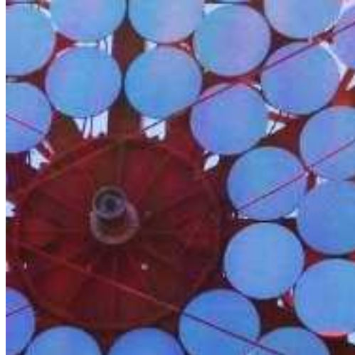
Figure 4.2: A picture of the lid CCD placed at the centre of each telescope.
