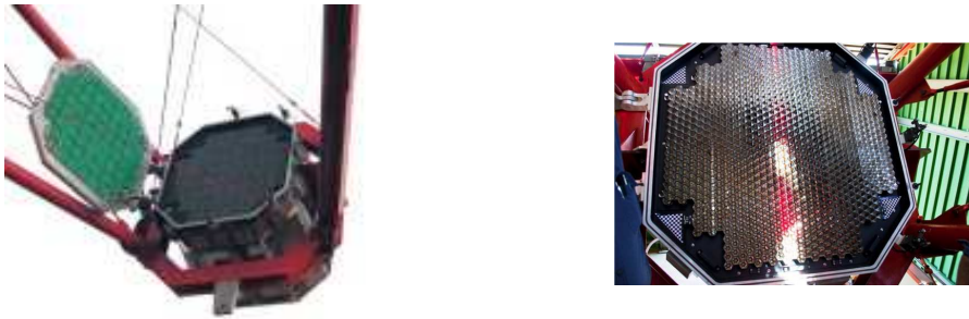
Figure 4.4: Left: The camera of a H.E.S.S. I telescope. Right: A close-up view of the H.E.S.S. II camera showing the photomultipliers and Winston cones
