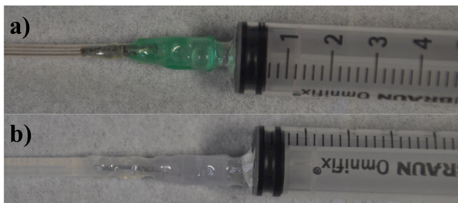
Figure 76: Images of the assembled pressure chambers used in CPA measurements for glass (a) and titanium (b) tubes. The use of quick-setting glue is illustrated, which was used to seal the syringe-needle and needle-tubing joints for a prevention of leakage during experiments.
