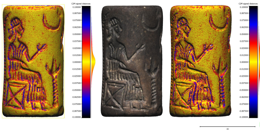
Figure 3. Comparing SFM to structured-light-scan. Left PhotoScan (RMS 0.028 mm), center the scan and right the VisualSFM (RMS 0.044 mm) model. The accuracy range is \pm 0.1 mm visualized by a morganstemming colorramp.
