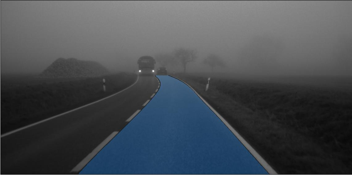
Figure 9.1: The pRSLC-based visibility estimation can be used as a fall-back solution for the RSLC-based algorithm proposed in Chap. 8, in cases of a partially obstructed road.
