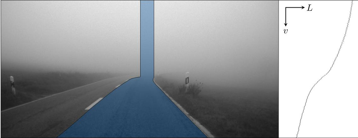
Figure 6.1: The road surface luminance curve (RSLC) is extracted line by line from the segmented region in the middle of the camera frame.
