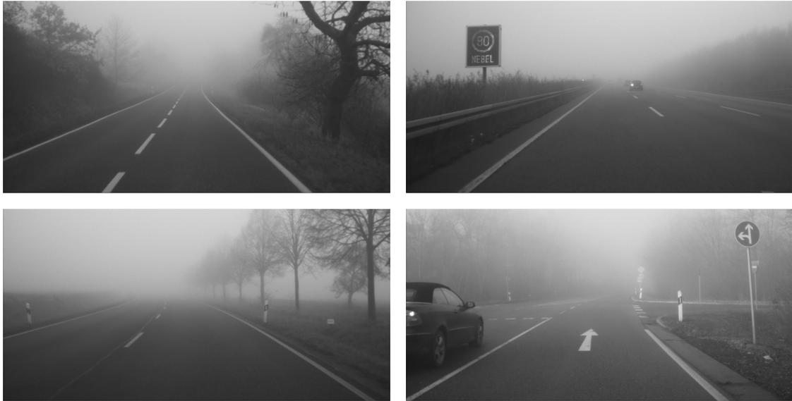
Figure 1.3: daytime fog captured by a driver assistance front camera
