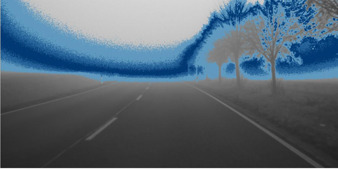
Figure 7.11: Highlighting of positions in a camera image that correspond to the  $L_{\text{air}}$  estimation. Dark blue: up to 5% relative difference, medium blue: up to 10% relative difference, light blue: up to 20% relative difference.
