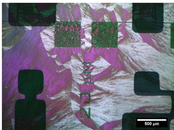
**Figure 107.** Optical microscopy image (almost crossed-polarisers) of a spin-cast film of **TIPS-PEN** from tetralin solution on polyimide coated glass FET-substrates with pre-structured bottom-contacts, Cytop™ dielectric and gate electrode.
