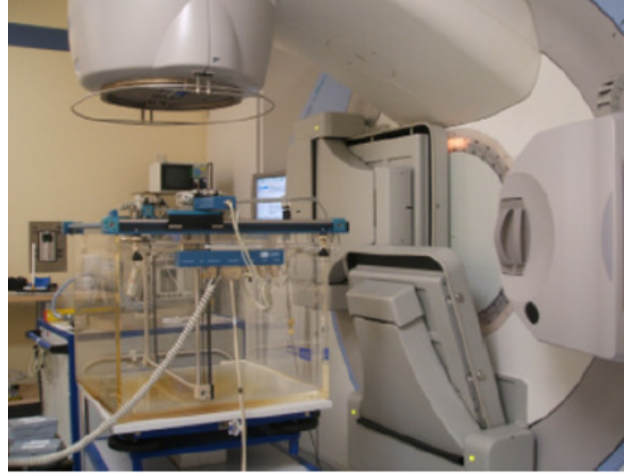
Figure 2.2: Measurement setup of the water tank to determine the beam quality for 6 MV linac (LINAC 1 ).
