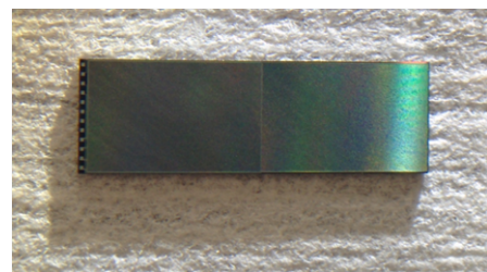
Figure 7.7.: Rectangular ISiPM die, with two ISiPM sensors, with total area of 15 \text{mm} \times 5 \text{mm} .
