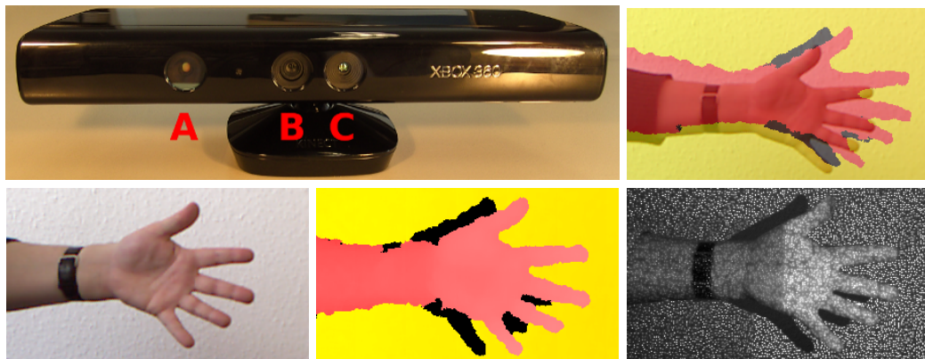
Figure 3.1.: Kinect device and its raw data output. Top: Kinect device with projector (A), color cam (B) and IR cam (C); color and depth channel overlaid. Bottom (left to right): raw color image; pseudo-color coding of the 11bit depth image provided by the on chip depth estimation; raw IR image showing the projected point pattern.
