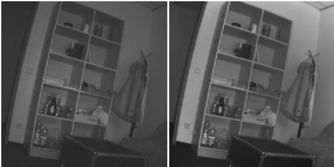
Figure A.3.: Raw intensity frame I_1 before ( left ) and after ( right ) homogenization. Like in Figure A.2, the fixed pattern noise (stripes introduced by tap reconstruction) is removed. Now the brightness even increases towards the edges. This is a slight over-correction because of different distance of the scene objects and the flat wall of the calibration frames but does not influence the flow computation.
