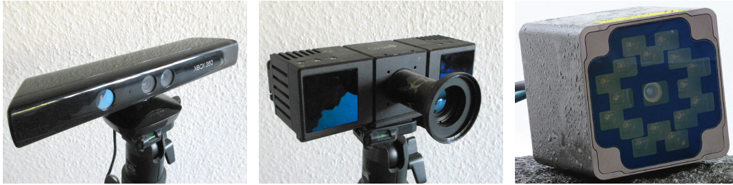
Figure 1.1.: Overview of the physical depth imaging devices used within this work: Microsoft Kinect ( left ), PMD CamCube3 ( center ) and Fotonix E40 ( right 1 )
