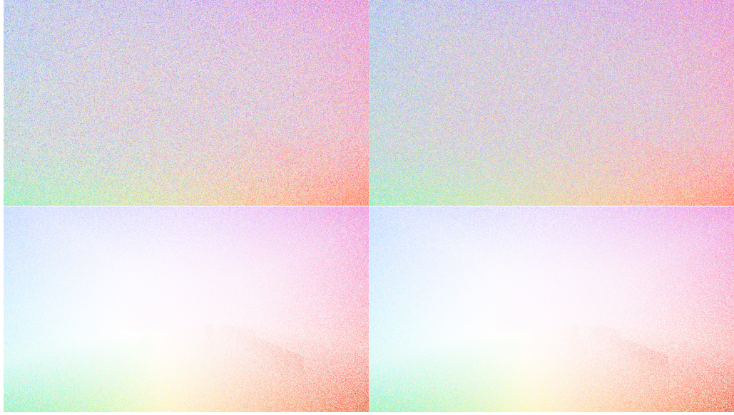
Figure 4.4: Different noise models for the observed data (optical flow, cf. Fig. 4.2): top left: additive Gaussian noise ( \mu = 0, \sigma^2 = 0.001 ), top right: additive uniform noise ( \mu = 0, \sigma^2 = 0.001 ), bottom left: multiplicative Gaussian noise ( \mu = 1, \sigma^2 = 1 ), bottom right: multiplicative uniform noise ( \mu = 1, \sigma^2 = 1 ).
