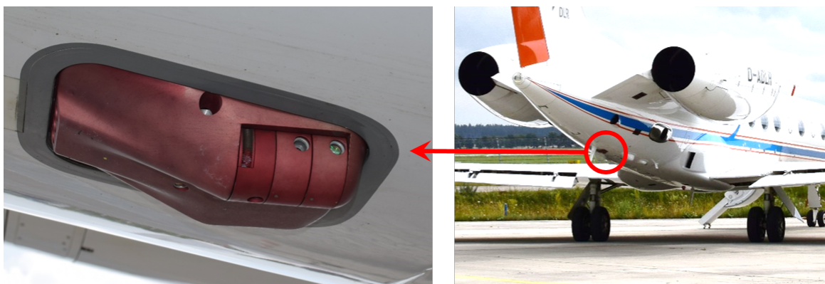
Figure 3.2: Image of the aperture plate mounted in the aircraft fuselage. The limb telescopes are pointing in starboard direction, perpendicular to the aircraft's main axis.
