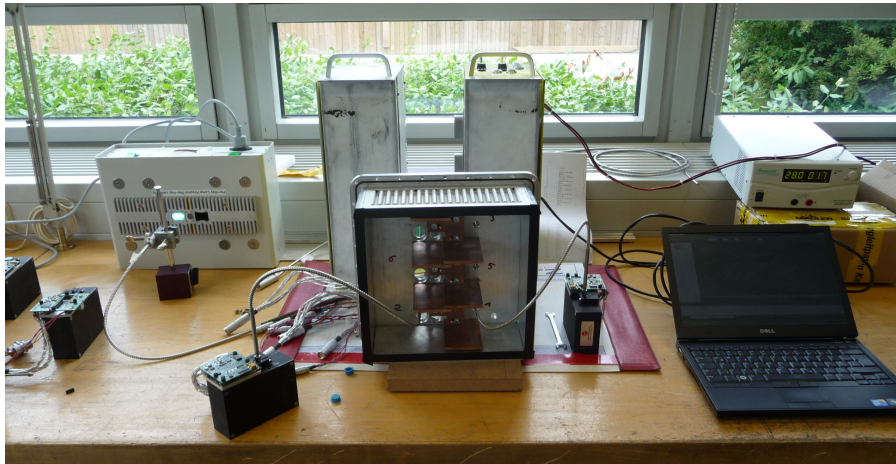
Figure A.4: Assembly of the spectrometer unit. Calibration gas lamp (Hg) on the left, spectrometer housing with opened bottom in the center, PC and electricity supply on the right. The fibre bundles are fixed to the spectrometer entrance slits while simultaneously controlling the slit function in order to optimise the imaging for each spectrometer.
