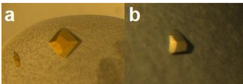
Figure 36: RosB crystals are shown, which are loaded with different flavins. a: RosB crystal loaded with AFP (orange), crystallization conditions: 0.3 M sodium formate, 0.1 M potassium chloride, 17 % (v/v) PEG 3350. b: RosB crystal loaded with HOC-RP, crystallization conditions: 0.3 M sodium formate, 25 % (v/v) Silver Bullet 49, 17 % (v/v) PEG 3350.
