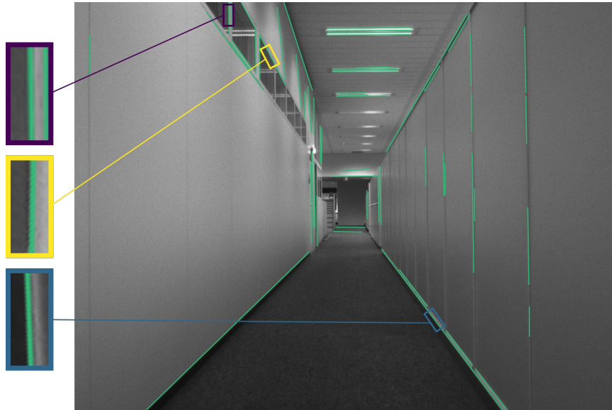
Figure 4.1.: Line segments separate homogeneous image regions. The surrounding neighborhoods are hence similar looking and the extracted descriptors not discriminative.
