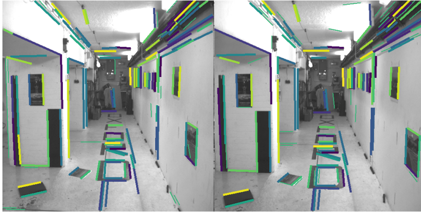
Figure 4.5.: Line matches generated with the optical flow line matching algorithm. Matching lines have the same color.
