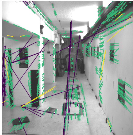
Figure 4.4.: Flow vectors in purple are discarded because of “appearance consistency”, flow vectors in yellow because they violate the “consistent motion constraint”. Only the flow vectors drawn in green are considered for further processing.
