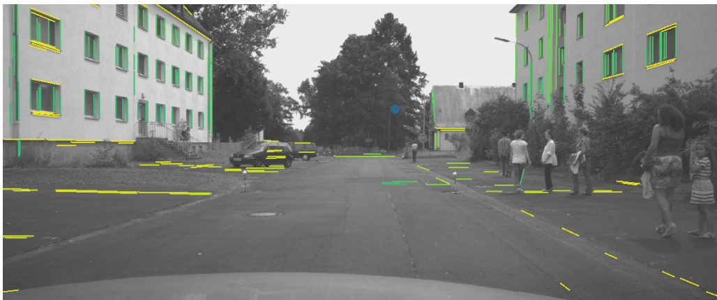
Figure 6.3.: Visualization of the angular distance from each line segment detected in the image to its corresponding epipolar line. The color indicates the angular distance, where yellow is "near" and green "far" from the epipolar line. The blue point marks the epipole.
