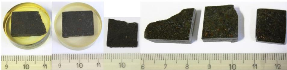
Figure 2.06: From left to right: NWA\_6966\_R (bombarded), NWA\_6966\_8 (non-bombarded), and remaining non-bombarded NWA 6966 pieces (4, 5, 6, 7) for applications of LSM, SEM and EMP. All targets are cut from one initial piece and got polished. Only the NWA\_6966\_R & NWA\_6966\_8 were embedded in epoxy.
