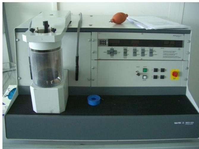
Figure 4.82: TEX MED 020 sputtering and vaporization device at the Institute of Earth Sciences at the University of Heidelberg.
