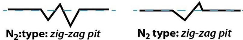
Figure 4.31: Sketch of other non-impact related  $N_2$  features, which are very small and found on non-bombarded and bombarded targets. Their profile shows a zig-zag pattern with major negative contribution.
