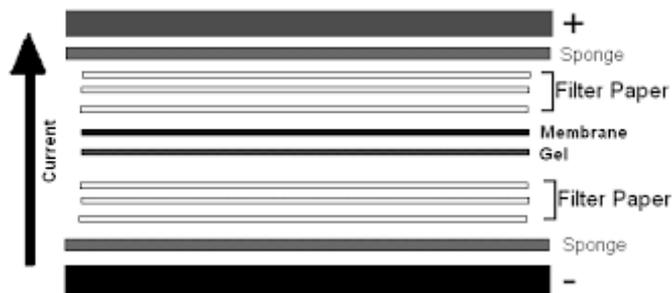
**Figure 2.2-2:** The gel-membrane sandwich
