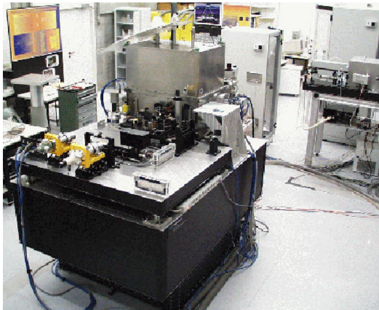
Figure 3.6: Scheme and overview of MIDI. In front of the dewar lies the Warm Optics bench. In the overview on the far right one can see the extra optical table carrying two of the three calibration light sources.
