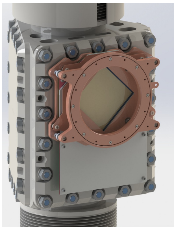
Figure 5.20: Drawing of the triangular detector chamber with the MOCCA detector placed on its holder. The figure was created by rendering a 3D model.
