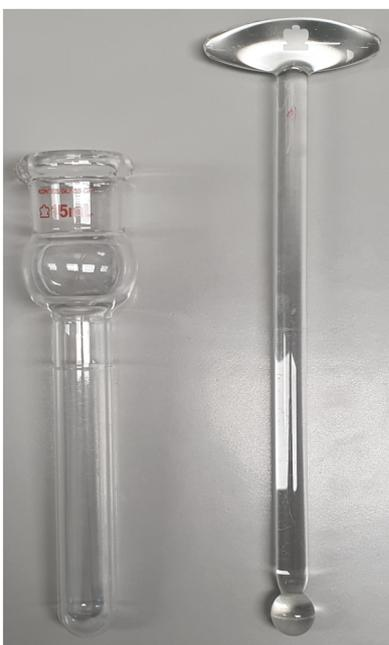
**Figure 4.3:** Dounce homogenizer used for sample preparation of porcine brain lysates. Tissue is forced through the small gap between the glass vessel (left) and the glass pestle (right) which mechanically disrupts cell membranes while leaving cell organelles intact.
