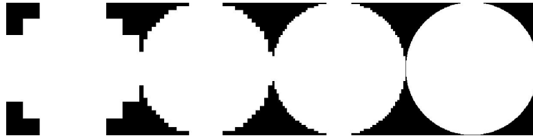
Figure 4.14: Pupil shape in the PD algorithm for three numbers of pixel used in the pupil sampling [8, 32, 64 and 256]. The oversampling factor of 2 in K band leads to corresponding image sizes equal to [32, 128, 256 and 1024].
