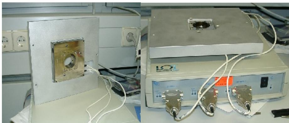
**Figure 11: The Queensgate nano positioning device NPS3330 XYZ**
