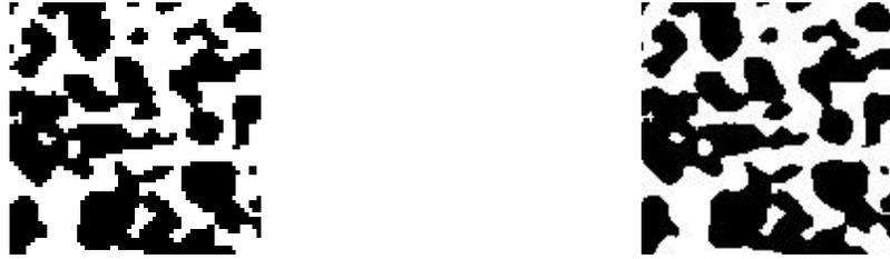
Figure 6.6: Cross section through the pore geometry of the medium P100. The image on the right hand side is a refinement due to a Shepard interpolation.
