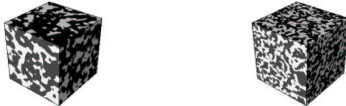
Figure 6.2: 3D visualization of the reconstructed pore geometry. On the left hand side P250 and on the right hand side P100. Both images show volumes of  $120^3$  voxel. Thus, the sample on the left hand side represents a volume of about  $47 \text{ mm}^3$  and the other a volume of about  $23 \text{ mm}^3$ .
