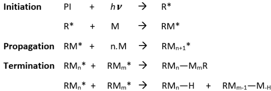
Figure 2.2: General process of free radical polymerization summarizing steps of initiation, propagation and termination. The schematic and caption are adapted from Fig.3 of [23].
