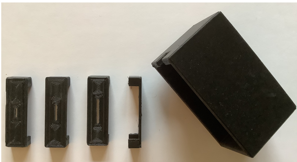
Figure 2.15: Image of 3D printed collimators with rectangular aperture sizes of 5.5 mm \times 1.8 mm, 15.5 mm \times 1.8 mm, 20.5 mm \times 1.8 mm, and 25.5 mm \times 1.8 mm along side with the lighth-tight cover.
