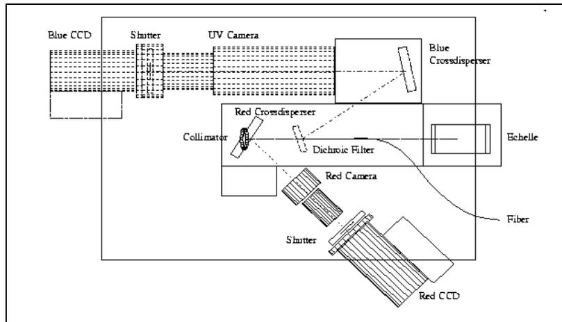
**Figure 2.2:** Schematic layout of FLASH (solid lines) respectively HEROS (with additional optical system, dashed lines). The light beam (long single dashes) enters the spectrograph by the optical fibre. After deflection at the echelle grating the beam is divided by a dichroic filter. The red light ( $\lambda > 5700 \text{ \AA}$ ) passes into the red channel (short dashes), the blue light is reflected into the blue channel (dashed dotted line).
