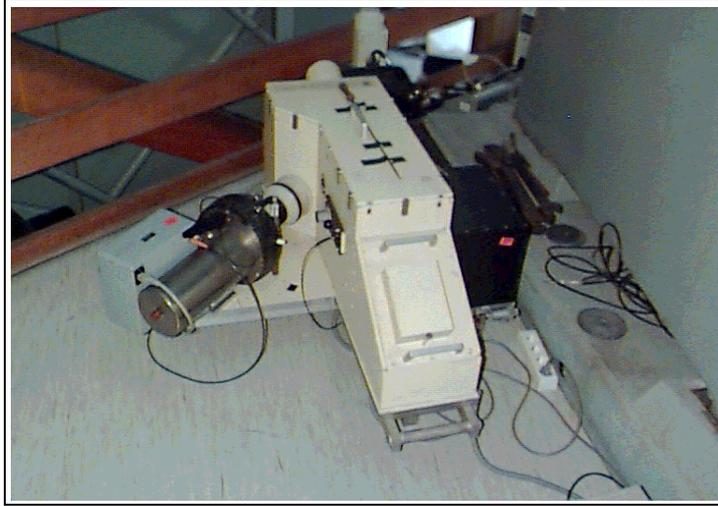
**Figure 2.1:** Echelle spectrograph HEROS. The former FLASH spectrograph consisting of the white box and the CCD system (small metal cylinder, attached to the left side of the box) constitutes the “red channel” of HEROS. HEROS is an upgrade of FLASH where a second optical system (the “blue channel”, the long black tube at the right side of the box) was added. The white box contains the optical fibre mounting, the collimator, the echelle grating, and the beam splitter.
