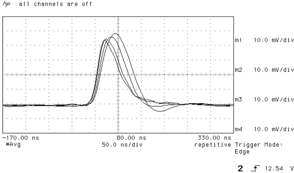
Figure 9.2: Impact of  $I_{sha}$  on Helix2.1-frontend’s pulse shape: from slowest to fastest pulse:  $I_{sha} = 60 \mu\text{A}$ ,  $100 \mu\text{A}$ ,  $200 \mu\text{A}$ , and  $300 \mu\text{A}$
