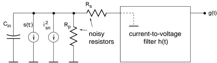
Figure 5.1: Filter with current-voltage transfer function  $h(t)$ ; parallel noise arises due to detector leakage shot-noise  $i_{sn}^2$  and  $R_p$ 's thermal noise, serial noise is caused by the thermal noise of  $R_s$ .
