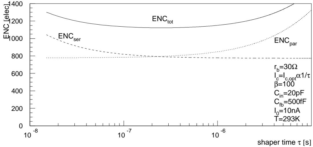
Figure 7.15: ENC (Equivalent noise charge) of the charge amplifier with bipolar input transistor with the parameters as given in the picture; the collector current is adapted to  $\tau$  to achieve optimum noise performance.
