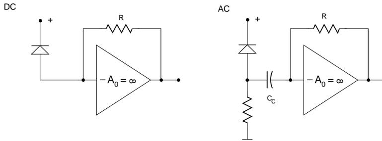
Figure 4.6: DC/AC-coupled photodiodes
