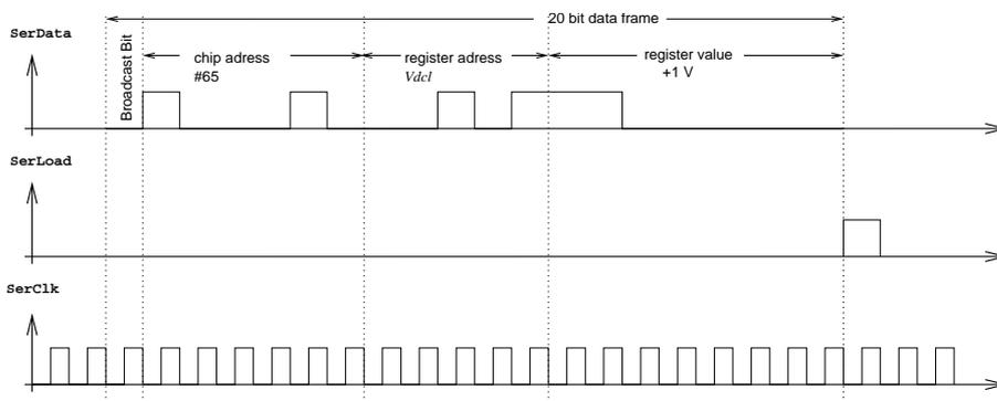
Figure D.16: Serial interface timing (Helix128S-2.0/2.1); substituting **SerClk** by **Rclk** and **SerData** by **TrigIn** gives the programming sequence of Helix128S-2.2/2.3. In the example plotted the *Vdcl* bias voltage is set to its nominal (Helix128-2.0/2.1/2.2) value of +1V.
