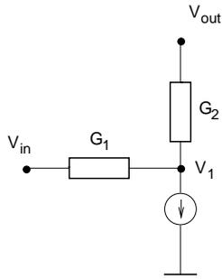
Figure 8.17: Large signal model of the shaper feedback network
