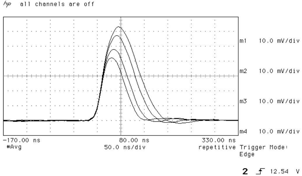
Figure 9.1: Impact of  $V_{fs}$  on Helix2.1-frontend’s pulse shape; from top to bottom:  $V_{fs} = 0.8$  V, 1 V, 1.5 V, and 2 V
