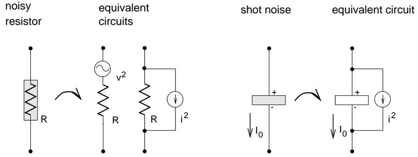
Figure 4.1: Equivalent circuit of noisy resistor (left) and of current shot noise (right)
