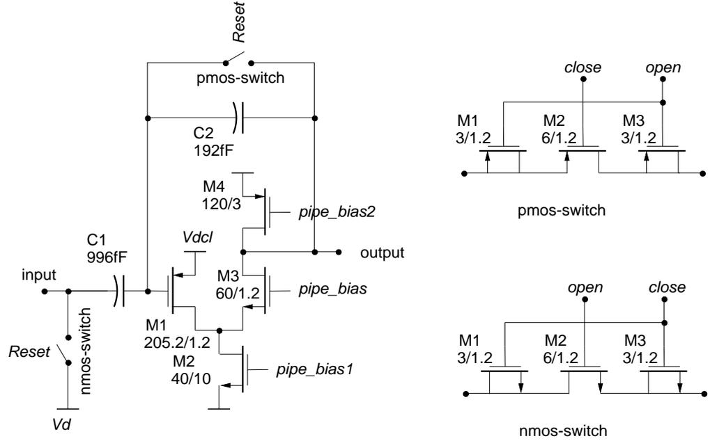
Figure 8.31: Detailed pipeline readout amplifier schematic; the pipeline readout amplifier is a resettable AC-coupled charge amplifier.
