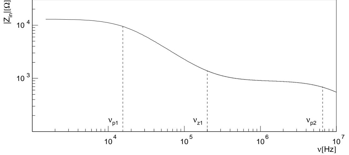
Figure 8.6: Bode-plot of input impedance; in the range between  $\nu_{p1}$  and  $\nu_{z1}$  the input impedance is capacitive with  $C_{in} = v_0 C_{fb}$ . For signal frequencies between  $\nu_{z1}$  and  $\nu_{p2}$  the input impedance is ohmic:  $R_{in} = \tau_2 / C_{in}$ .
