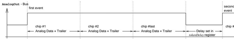
Figure D.14: Analog current signal on the AnalogOut bus for the daisy chain illustrated in fig. D.13
