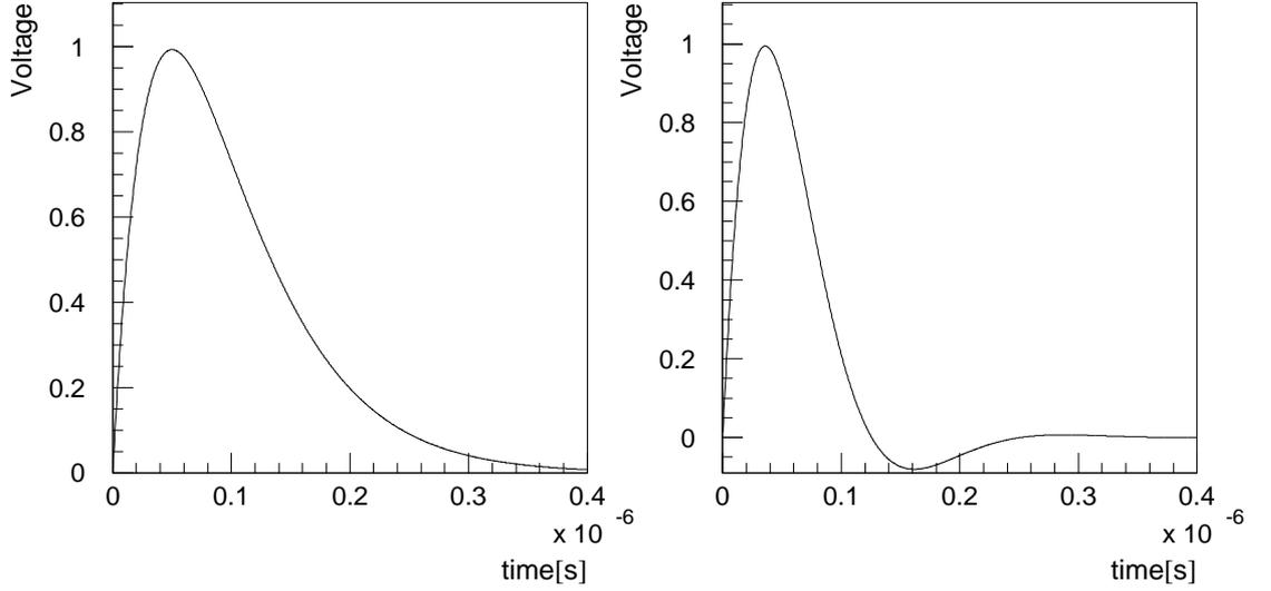
Figure 8.13: Left: ideal semi-gaussian pulse  $v_{out}(t) = te^{-\beta t}$ ; right: pulse shape with undershoot  $v_{out}(t) = \frac{1}{\alpha} \sin(\alpha t)e^{-\beta t}$  ( $\alpha=1/50\text{ns}$ ,  $\beta=1/40\text{ns}$ )
