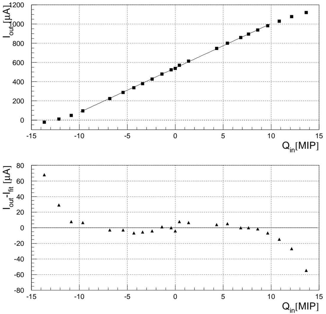
Figure 9.7: Measured linearity of HELIX128S-2 at low Sclk-frequency
