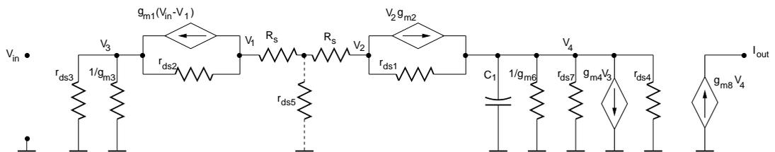
Figure 8.37: Small signal model of current buffer
