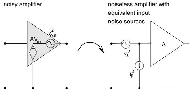
Figure 4.2: Noisy amplifier can be modelled by a noiseless amplifier and two equivalent input noise sources.
