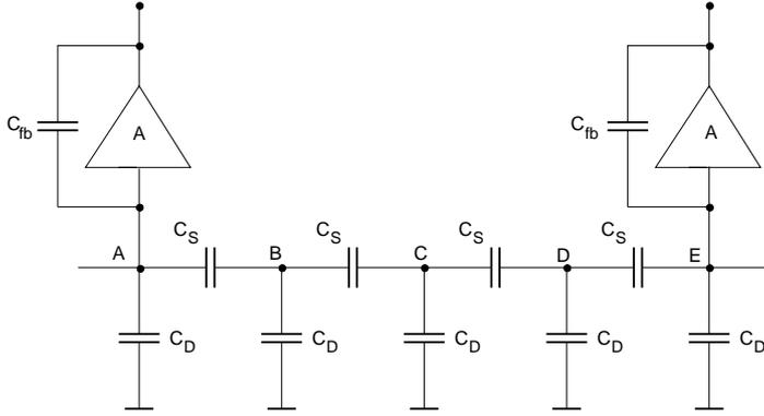
Figure 2.5: Capacitive charge sharing: every 4th strip is connected to a charge amplifier with input capacitance  $A \cdot C_{fb}$ . If a charge  $Q$  is put on node B, mirror charges can be obtained at nodes A and E where  $Q_A/Q_E=3$ .  $Q_A + Q_E < Q$  due to “charge loss” on the  $C_D$ 's [Bau90].
