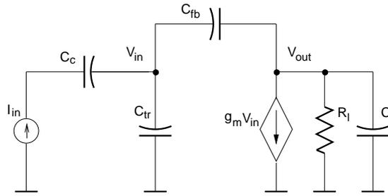
Figure 8.30: Small signal model of pipeline readout amplifier
