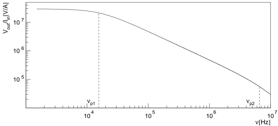
Figure 8.4: Bode-plot of transfer function  $v_{out}/i_{in}(\nu)$ ; in the range between  $\nu_{p1}$  and  $\nu_{p2}$  the preamp integrates current. The gain is given by  $v_{out} = i_{in}/(sC_{fb}) = q_{in}/C_{fb}$ .
