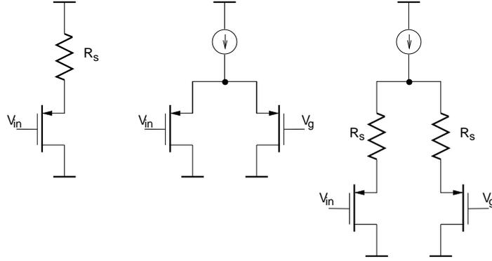
Figure 8.38: Left: transistor with source degeneration (source follower configuration); the source resistance “linearizes” the square law voltage-current relation of the MOSFET. Middle: differential transistor stage; the differential configuration also enhances linearity. Right: differential transistor stage with source degeneration for optimum linearity
