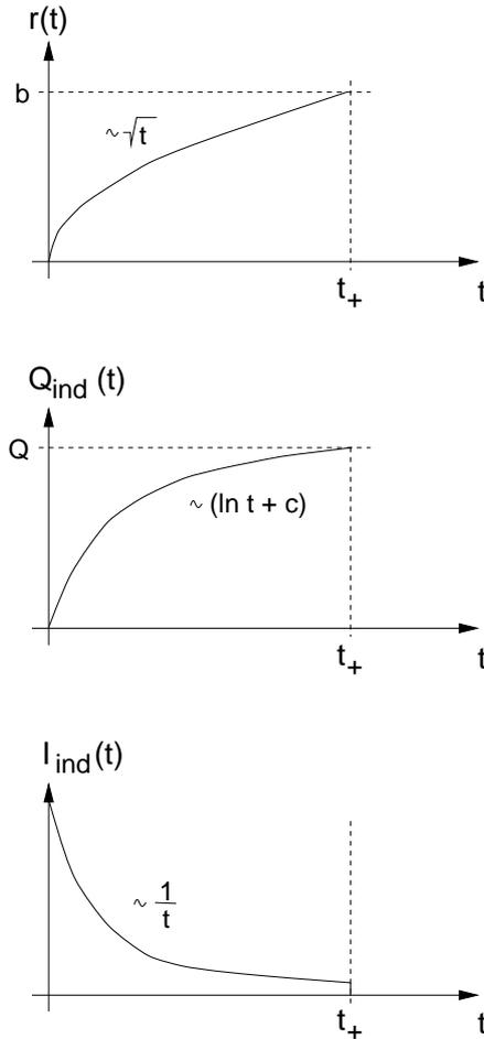
Figure 3.1: Drift of a positive ion  $Q$  in a cylindrical proportional counter: path  $r(t)$ , induced charge  $Q_{ind}(t)$ , and induced current  $I_{ind}(t)$  vs. time
