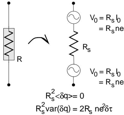
Figure 5.4: A (serial) noisy resistor is modelled by a noiseless resistor with two antiparallel voltage sources in series, which have equal mean voltages. The variance of the voltage-time products per time slot  $[\tau, \tau + \delta\tau]$  of each voltage source is  $R_s^2 \text{var}(\delta q) = R_s^2 n e^2 \delta\tau$ .
