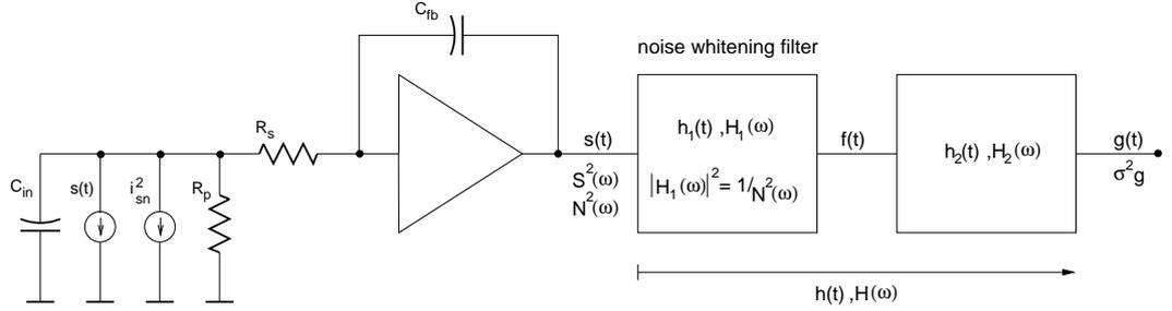
Figure 6.13: Signal processing architecture for optimum signal processing
