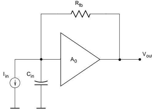
Figure 7.2: Current amplifier with capacitive source impedance
