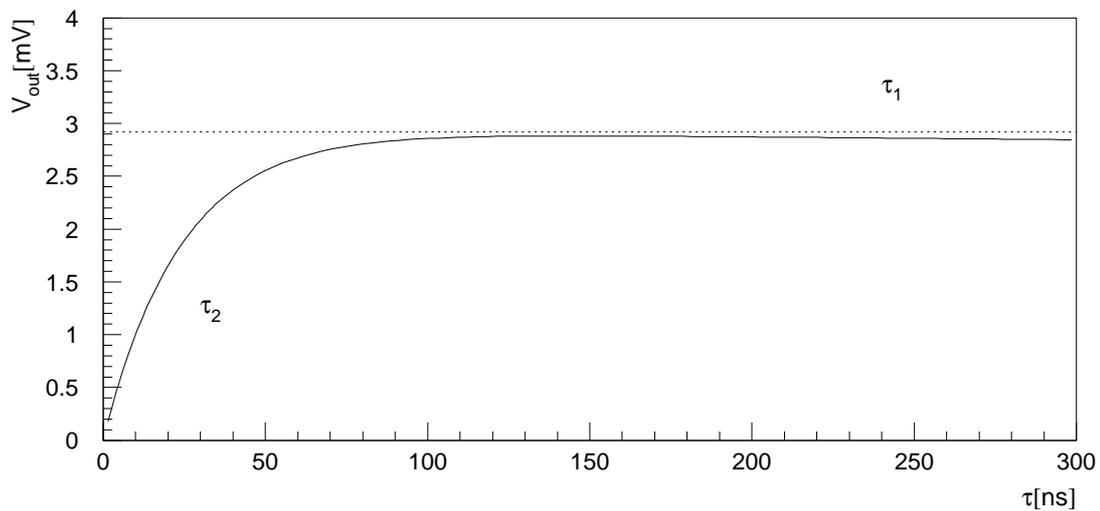
Figure 8.5: Preamplifier response to a  $\delta$ -like current pulse of 1fF charge; the rise is determined by  $\tau_2$ .  $\tau_1$  is the time constant of the exponential discharge of the feedback resistor  $C_{fb}$  via  $R_{fb}$ .
