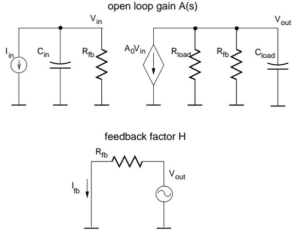
Figure 7.6: Current amplifier with single-pole open-loop gain cell
