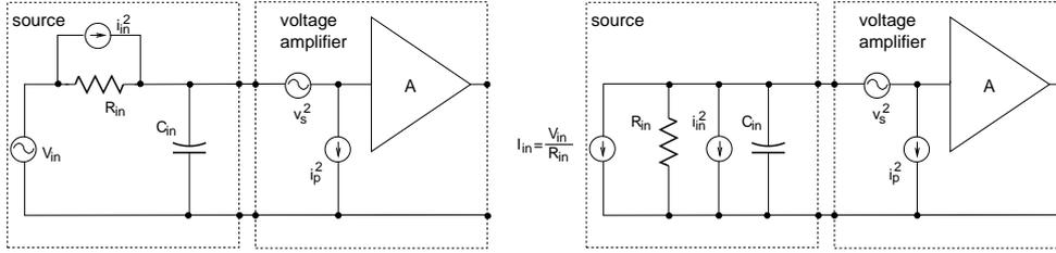
Figure 4.4: Left: voltage amplifier with resistive and capacitive signal source; right: the voltage source has been transformed into a current source.
