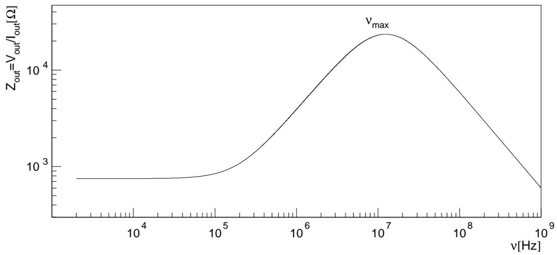
Figure 8.19: Bode-plot of the shaper output impedance  $v_{out}/i_{out}(\nu)$
