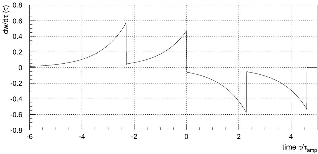
Figure 6.9: Weighting function  $w(\tau)$  and its derivative  $\dot{w}(\tau)$  vs. time  $\tau$  of signal arrival for quadruple correlated voltage sampling at charge amplifier output
