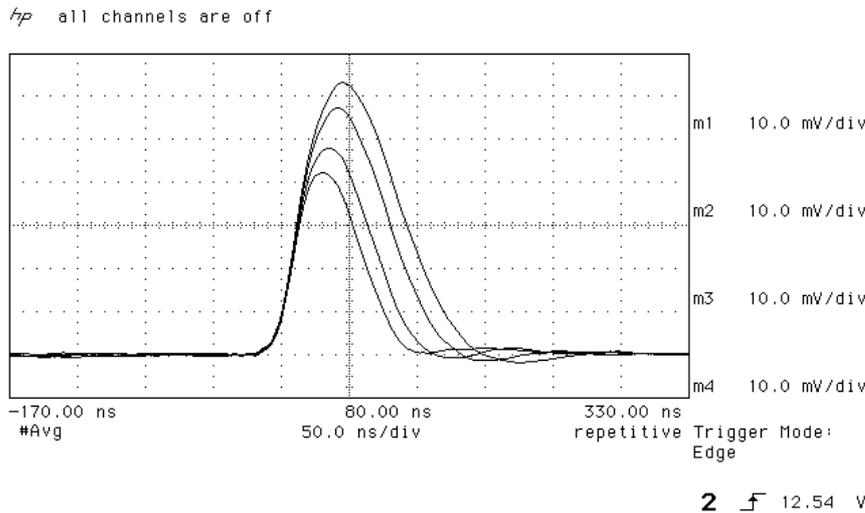
Figure D.4: Impact of  $V_{fs}$  on pulse shape: from outside to inside  $V_{fs}=0.8\text{V}, 1\text{V}, 1.5\text{V}$ , and  $2\text{V}$
