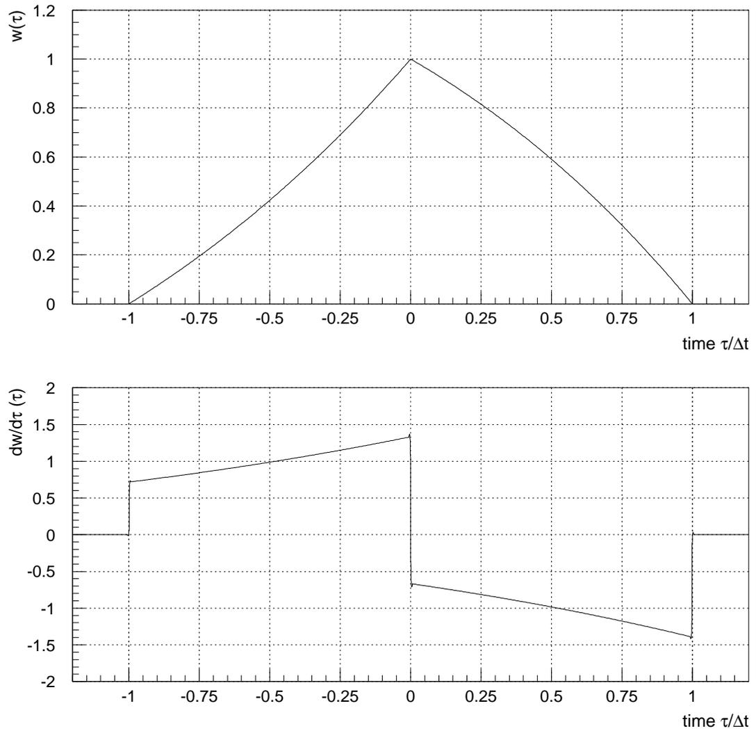
Figure 6.12: Weighting function  $w(\tau)$  and its derivative  $\dot{w}(\tau)$  vs. time  $\tau$  of signal arrival for deconvolution of CR-RC-shaping;  $\Delta t$  denotes the sampling interval. The peak of the shaped pulse takes place at  $T_{peak}=3\Delta t$  [RD20-2].
