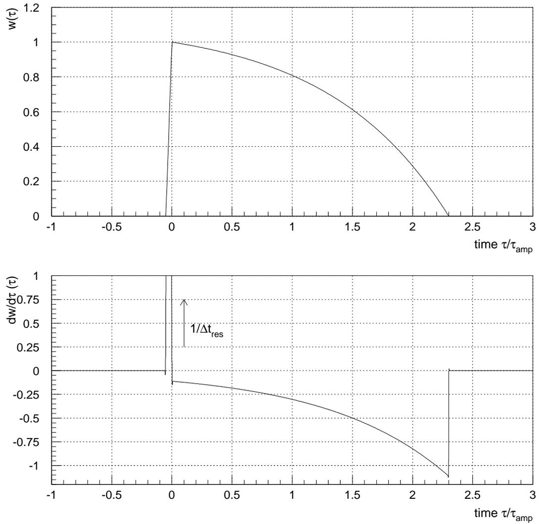
Figure 6.2: Weighting function  $w(\tau)$  and its derivative  $\dot{w}(\tau)$  vs. time  $\tau$  of signal arrival for single voltage sampling with reset. For  $\Delta t_{res} \rightarrow 0$  the dotted weighting function becomes infinite at  $\Delta t_{res} < \tau < 0$ .
