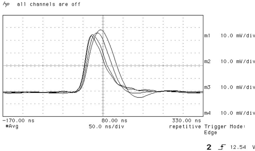
Figure D.3: Impact of  $I_{sha}$  on pulse shape: from slowest to fastest pulse:  $I_{sha}=60\mu\text{A}, 100\mu\text{A}, 200\mu\text{A}$ , and  $300\mu\text{A}$
