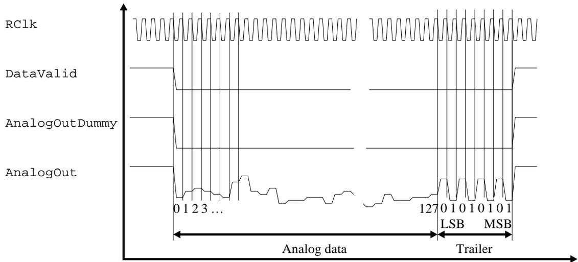
Figure D.9: Format of a readout burst
