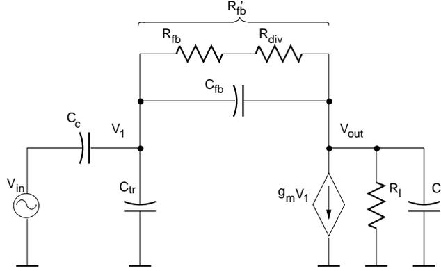
Figure 8.11: Small signal model of shaper; the actual values taken from the SPICE model 2 are given in table 8.3.
