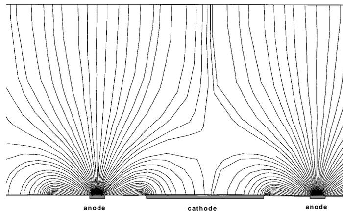
Figure 3.3: Electrical field inside a MSGC [Bre97]: electrons/ions move along the field lines to the electrodes. The densely spaced field lines around the anodes indicate a high field strength.
