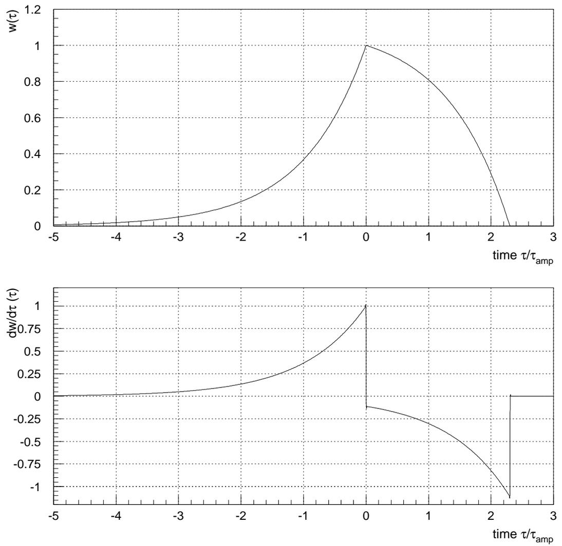
Figure 6.6: Weighting function  $w(\tau)$  and its derivative  $\dot{w}(\tau)$  vs. time  $\tau$  of signal arrival for double correlated voltage sampling
