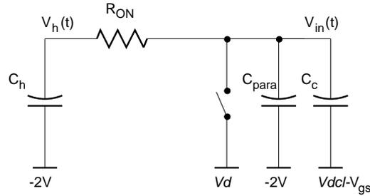
Figure 8.29: Capacitances attributed to the read-line;  $C_c$  is connected to the “virtual ground” of the pipeamp ( $\approx Vdcl - V_{gs}$ ).  $Vd$  is the reset potential.
