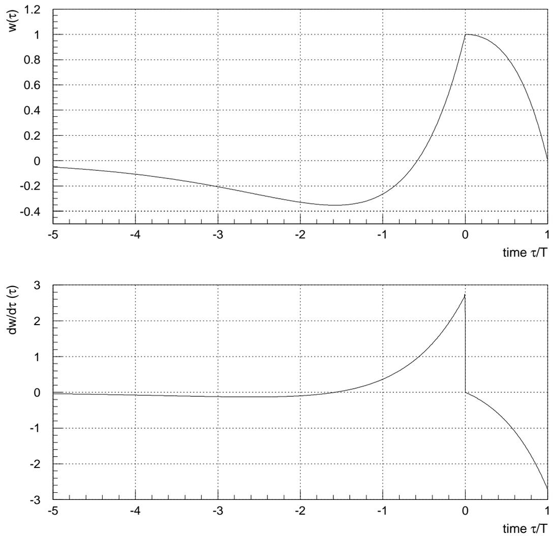
Figure 6.8: Weighting function  $w(\tau)$  and its derivative  $\dot{w}(\tau)$  vs. time  $\tau$  of signal arrival for double correlated sampling behind CR-RC-shaper
