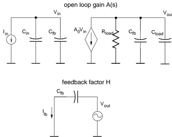
Figure 7.11: Charge amplifier with capacitive source and pole at the amplifier output
