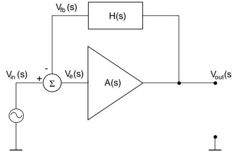
Figure 7.1: Basic feedback circuit
