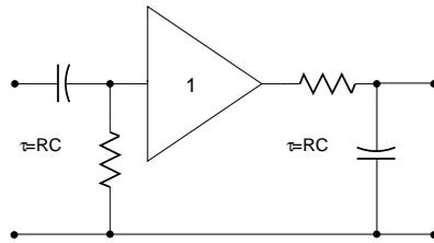
Figure 4.9: CR-RC-band pass filter which forms (“shapes”) the signals behind the charge amplifier
