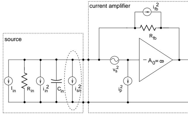
Figure 4.5: Current amplifier; the source is modelled as an ideal current source with a resistive and capacitive output impedance in parallel.  $i_{sn}^2$  denominates the shot noise of a photodiode's leakage current.
