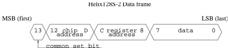
Figure D.15: Data format of the Helix128-2 chip
