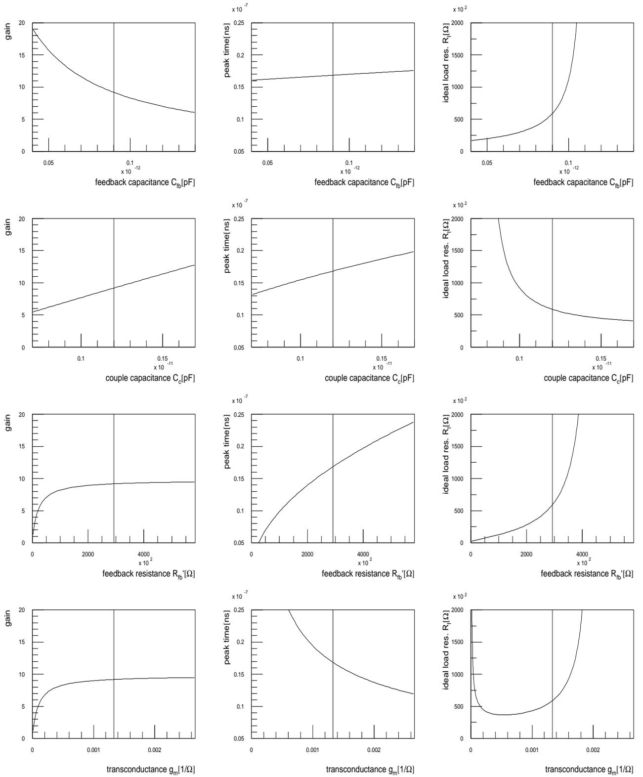
Figure 8.14: Dependency of shaper gain, peak time, and ideal load resistance on feedback capacitance  $C_{fb}$ , couple capacitance  $C_c$ , feedback resistance  $R_{fb}$  and input transistor transconductance  $g_m$ ; vertical lines indicate the chosen design value.
