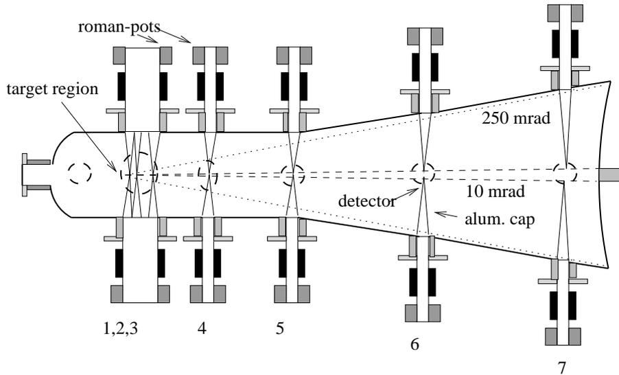
Figure 1.5: Silicon vertex detector tank [Knö95]
