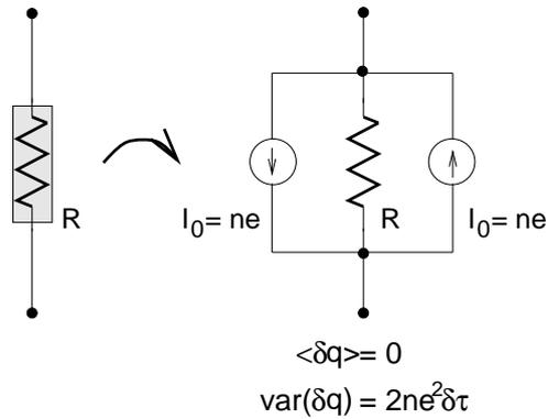
Figure 5.3: A (parallel) noisy resistor is modelled by a noiseless resistor with two antiparallel current sources with equal mean currents. The variance of charge per time slot  $[\tau, \tau + \delta\tau]$  of each current source is  $\text{var}(\delta q) = ne^2\delta\tau$ .
