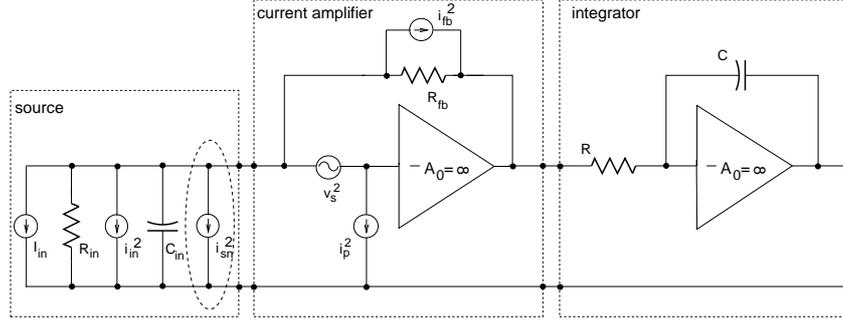
Figure 4.7: Current amplifier with subsequent integrating stage
