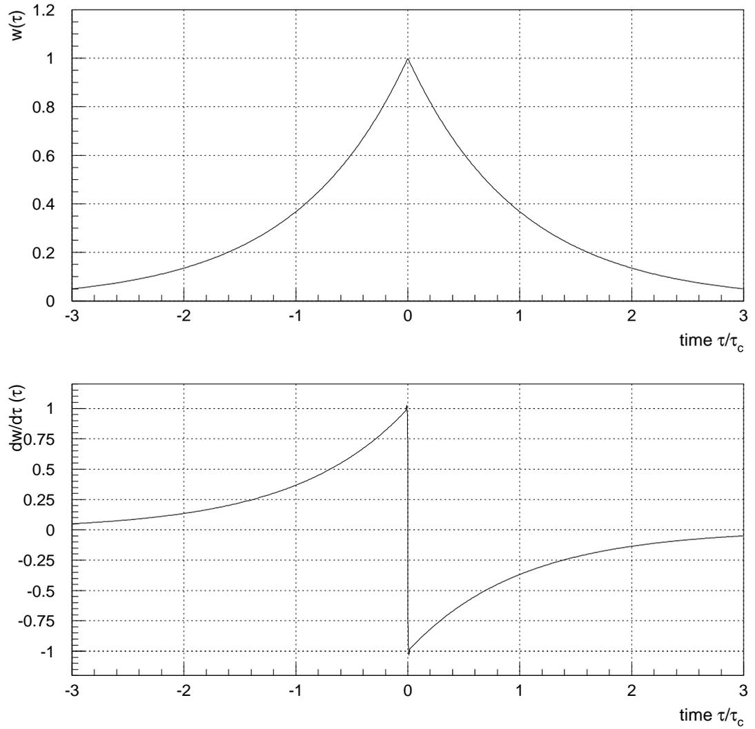
Figure 6.14: Weighting function  $w(\tau)$  and its derivative  $\dot{w}(\tau)$  vs. time  $\tau$  of signal arrival for optimum filter (“cusp”).  $\tau_c$  denotes the time constant of the noise-whitening CR-filter.
