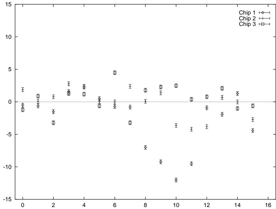
Figure 9.4: Comparator offset variations measured on three IDEFIX test chips with 16 channels each [Gla97]
