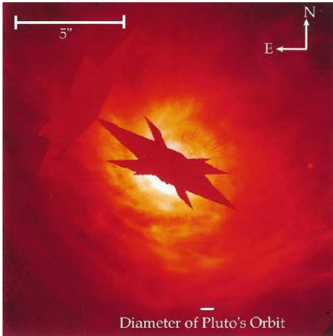
Figure 3.6: Hubble Space Telescope STIS coronagraphic image of the circumstellar environment of AB Aur, co-added from two images obtained with different instrument rotations. The irregular polygons are portions of the field that were occulted by the STIS wedge structure or the diffraction spikes in both observations. From Grady et al. (1999b).
