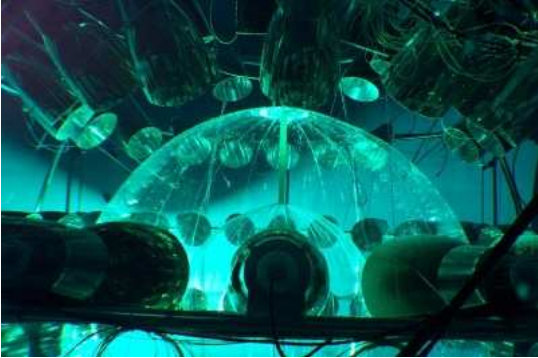
Figure 4.2: The inner and outer vessels in the CTF open structure.
