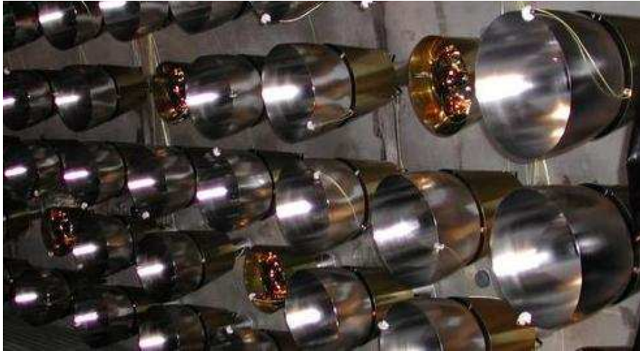
Figure 2.7: A closeup view of the Borexino photomultiplier tubes (PMT's). On the PMT's equipped with the light concentrator is visible the thin fiber for the calibration of the pulse time and gain response.
