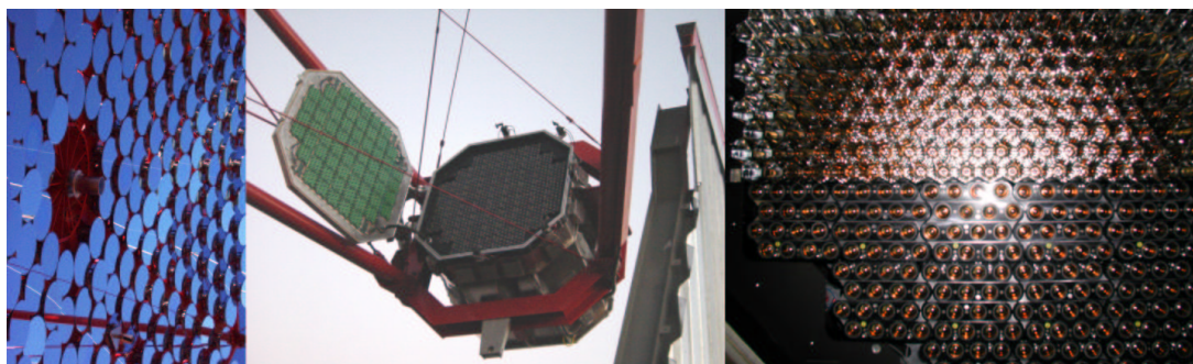
Figure 2.9: Left: Close-up view on the mirrors of a H.E.S.S. telescope. Middle: The camera of one H.E.S.S. telescope with open lid. Right: Close-up view on the photomultipliers and Winston cones of the first H.E.S.S. camera.
