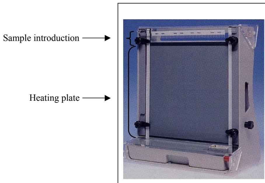
Figure 29. Sequencing gel chamber from GIBCO BRL used for electrophoresis of both thin (0.4 mm) and thick (1.0 mm) gels. Picture taken from the website of GIBCO BRL.
