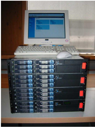
FIGURE A.1: Photograph of the production quality system of a Distributed RAID. The lower three nodes (backends) have local hardware RAIDs, each of which comprises six 200 GB SATA disk drives (five data disks and one spare device). The upper node is used as the frontend, which imports the remote devices via ENBD. In this specific configuration, the total raw capacity of the system is 3.6 terabytes.
