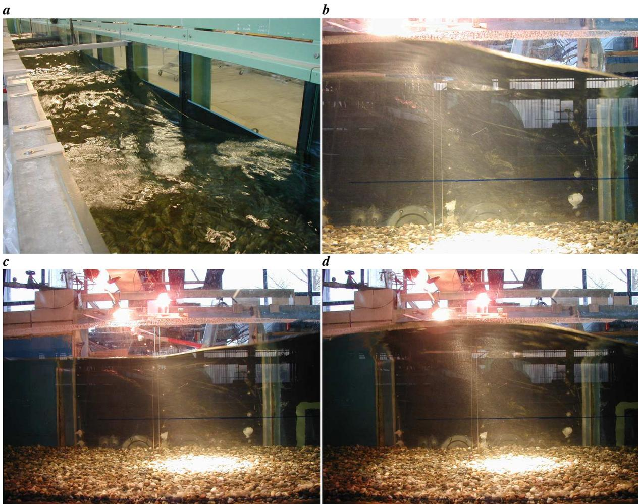
**Figure 10.4:** Wave experiments. *a* Surface waves propagating along the channel. *b*, *c*, *d* Three successive images of a surface wave passing the observation area. These images also show a basic limitation of the free surface flow setup: the bright light scattering at the gravel surface. Further, the instationary water surface is responsible for large illumination inhomogeneities due to refraction.
