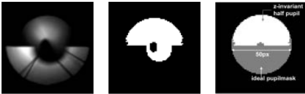
Figure 4.27: Left: Resulting signal in the PIGS/z-invariant WFS-camera after placing a half mask into the exit pupil. The upper half shows flux resulting from reflections by the rod. Middle: Binary mask to highlight parts of the re-imaged pupil, which are suitable for further data processing. Right: The diameter of the re-imaged pupil was estimated in pixel by superimposing a circular pupil.
