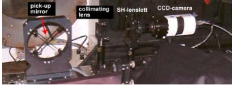
Figure 4.15: Image of the SHS reference setup. From left to right: Pickup mirror collimator lens, SH-lenslet and objective with Retiga 2000 CCD-camera.
