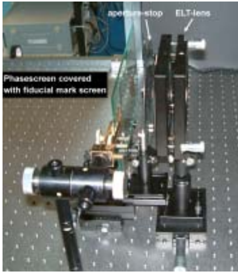
Figure 3.3: Atmosphere and telescope simulator. From left to right: phase screen, aperture stop and ELT-lens.
