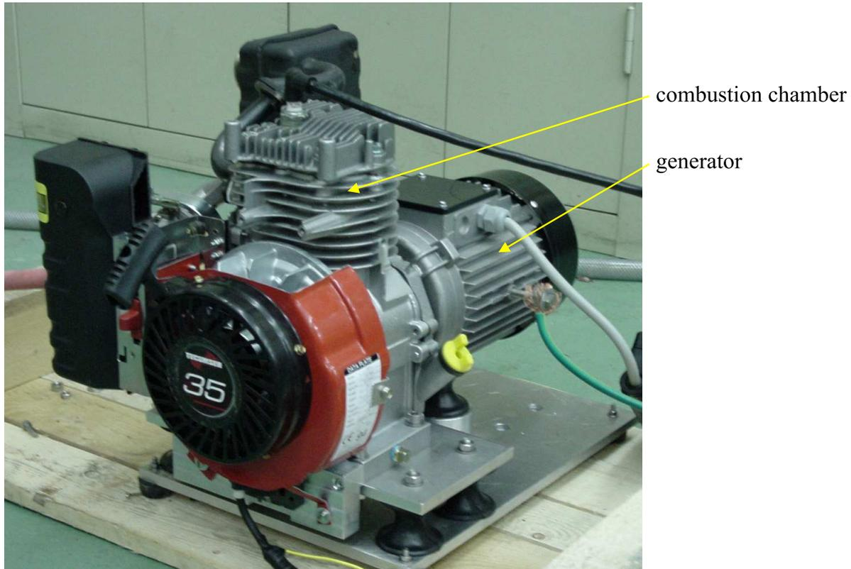
**Figure 6.5:** Power generator with carburetor engine
