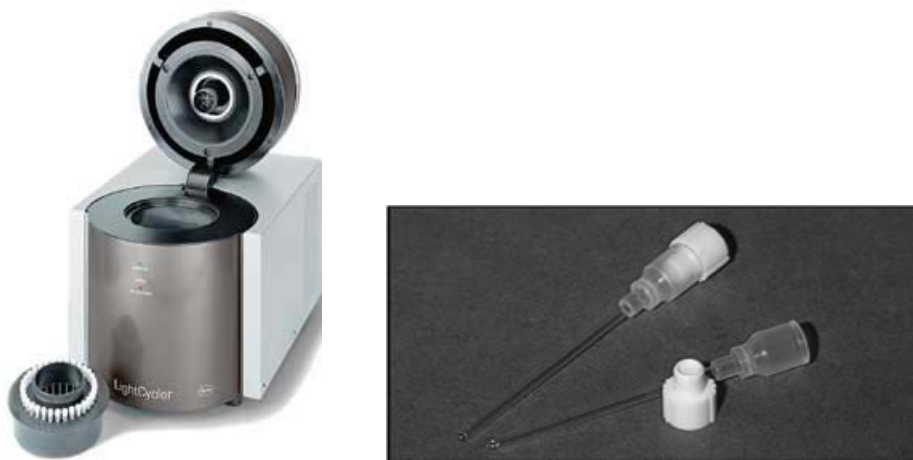
Fig.35 LightCycler ® Instrument with sample carousel. PCR occurs in specially designed borosilicate glass capillaries (Roche).
