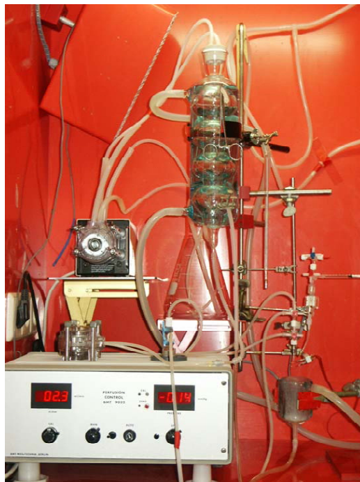
Fig.19 A complete Langendorff apparatus. Temperature controlled perfusion chamber maintains inner temperature of 38°C.
