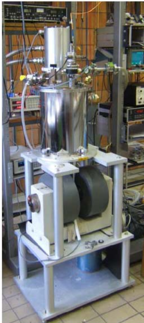
Figure 69: Photograph of the cryostat with attached magnetic coils used for magnetoresistance measurements as a function of T at the EPFL in Lausanne.
