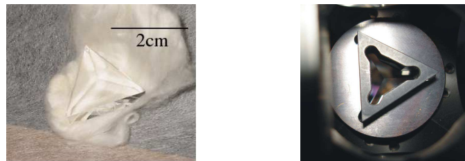
Figure 6.7: Topview on the tip of the 3-sided pyramid prism, unmounted and in its holder.
