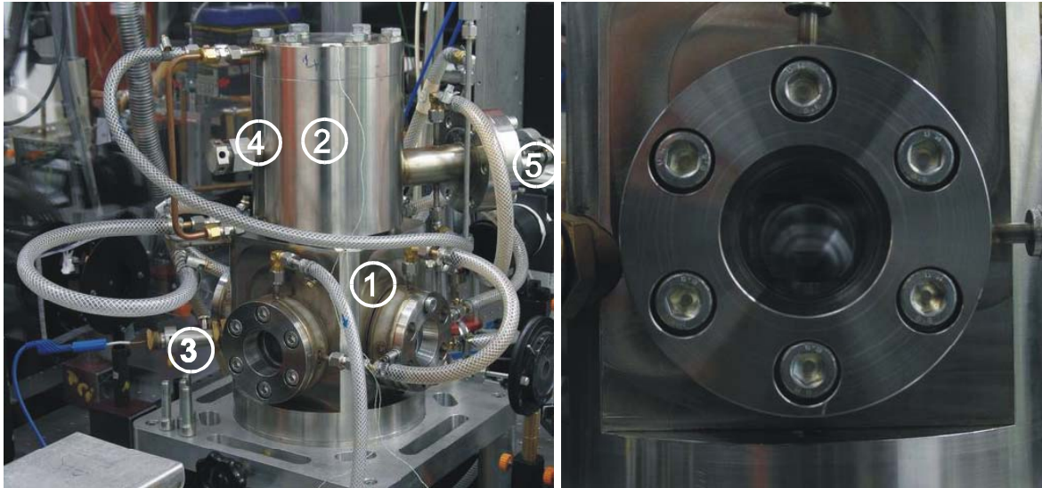
Figure 4.2. The high-pressure burner (left): 1) Burner housing 2) Heat exchanger 3) Ignition device 4) pressure relief valve 5) exhaust. One of four windows for optical access (right).
