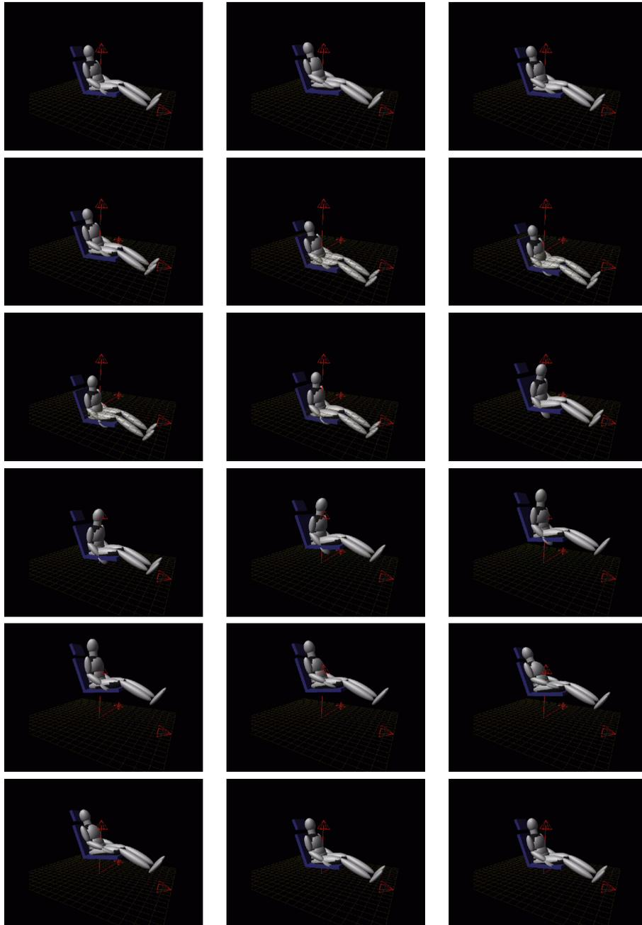
Figure 14.2: Snapshots of a human in a seat with a strong vertical excitation (Please, look at the pictures line for line.)
